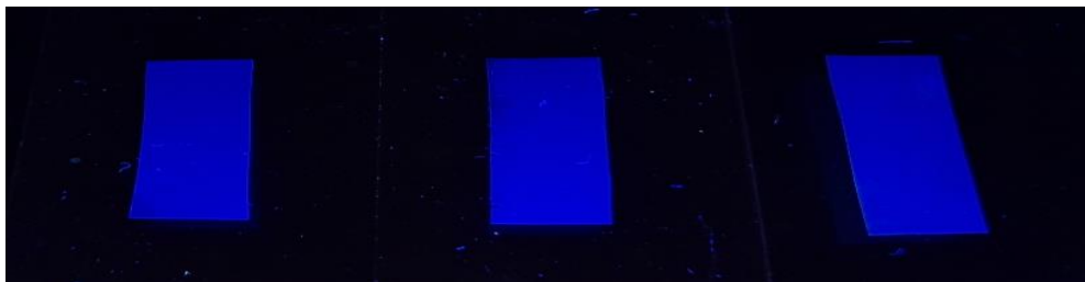
Figure 4.7: Photograph of compounds 3-5 in 2% PMMA film under handheld UV lamp irradiated at 365 nm.
