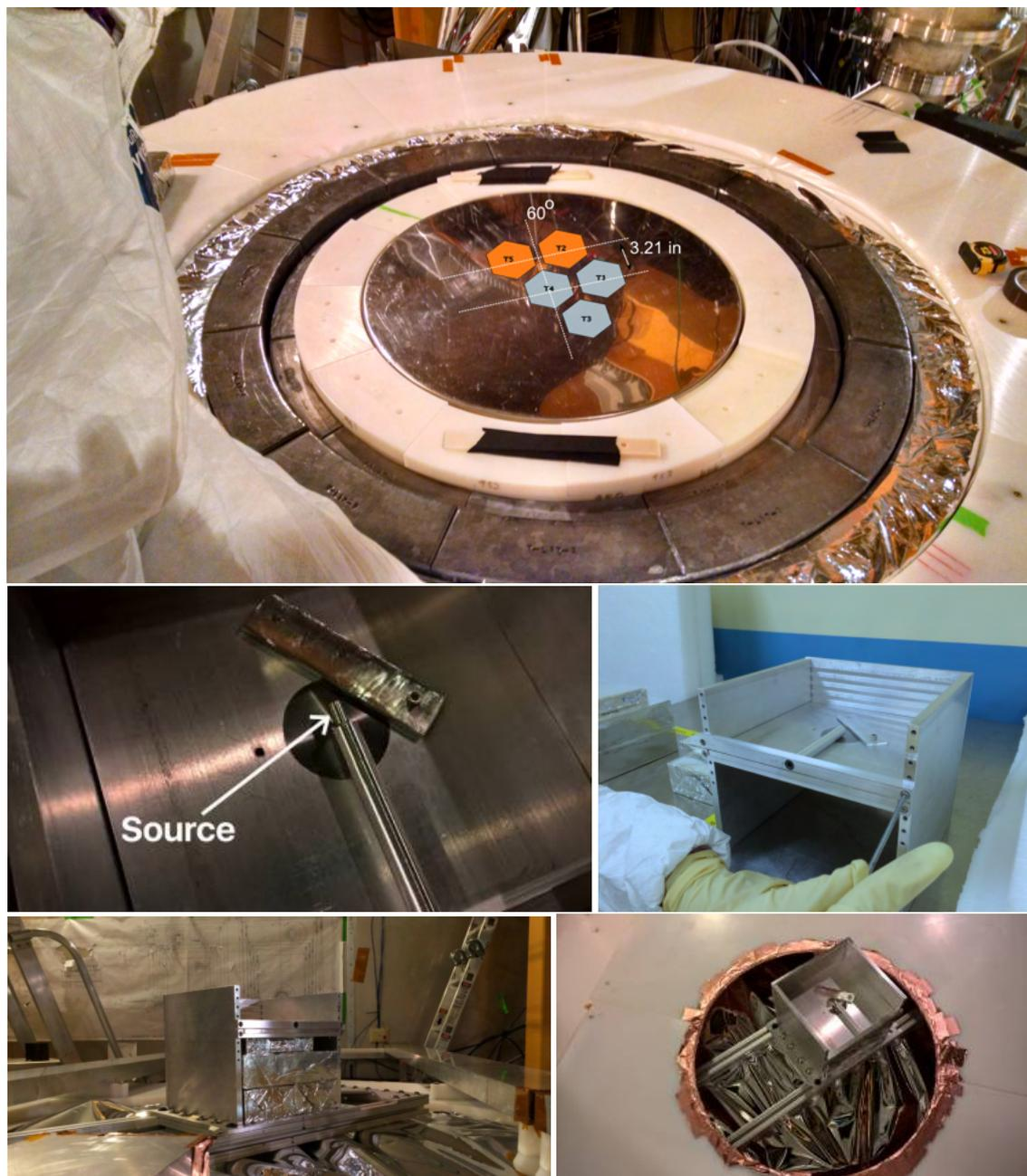
FIGURE 3.5: (a) Top view of the SuperCDMS Soudan ice box, (b) top view of the gamma source rod with the  $^9\text{Be}$  wafer underneath. The gamma source is placed within the source rod, (c) the source box with the detachable source rod, (d) side view of the source box with the lead shielding to counter the high gamma rate from the source, and (e) top view of the source box placed on a bridge above detector towers 2 and 5.
