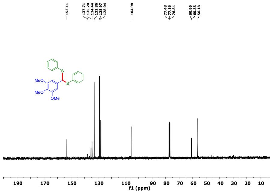
Figure 5.54. <sup>13</sup>C NMR spectrum of ((3,4,5-trimethoxyphenyl)methylene)bis(phenylsulfane)
