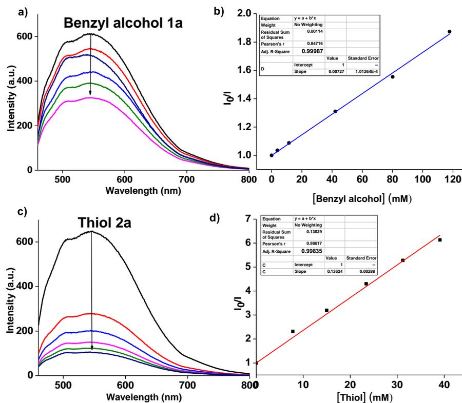
**Figure 5.6.** a) Fluorescence quenching of catalyst by benzyl alcohol **1a**; b) Stern-Volmer plot of **1a**; c) Fluorescence quenching of catalyst by thiophenol; d) Stern-Volmer plot of **2a**.
