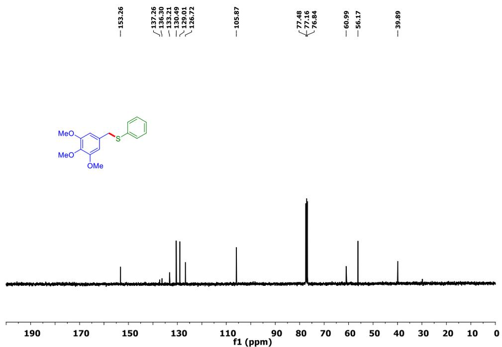
Figure 5.52. <sup>13</sup>C NMR spectrum of phenyl(3,4,5-trimethoxybenzyl)sulfane (**4qa**)
