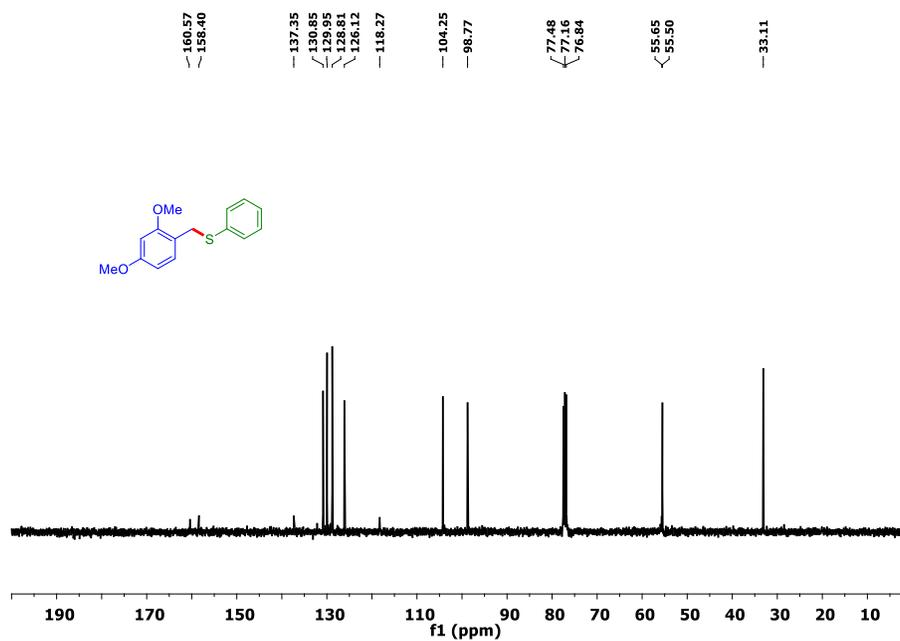
Figure 5.42. <sup>13</sup>C NMR spectrum of (2,4-dimethoxybenzyl)(phenyl)sulfane (**4na**)
