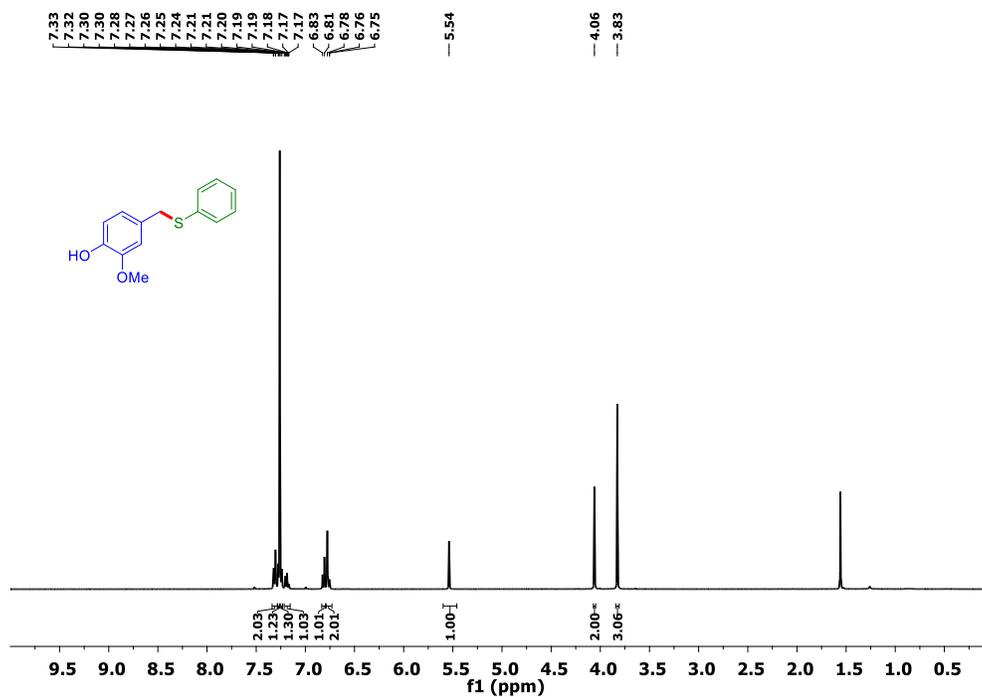
Figure 5.57.  $^1\text{H}$  NMR spectrum of 2-methoxy-4-((phenylthio)methyl)phenol (4sa)
