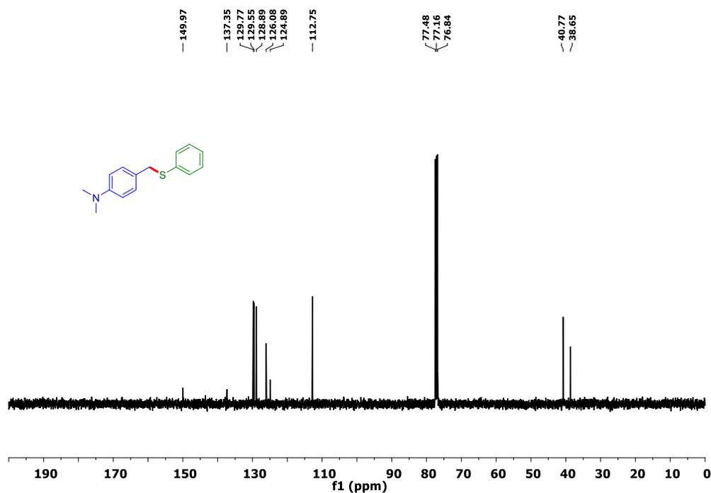
Figure 5.56. <sup>13</sup>C NMR spectrum of N,N-dimethyl-4-((phenylthio)methyl)aniline (4ra)
