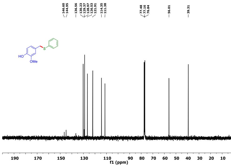
Figure 5.58.  $^{13}\text{C}$  NMR spectrum of 2-methoxy-4-((phenylthio)methyl)phenol (4sa)
