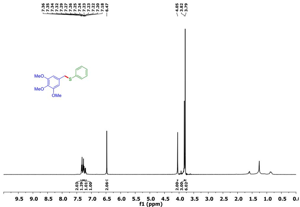
Figure 5.51. <sup>1</sup>H NMR spectrum of phenyl(3,4,5-trimethoxybenzyl)sulfane (**4qa**)
