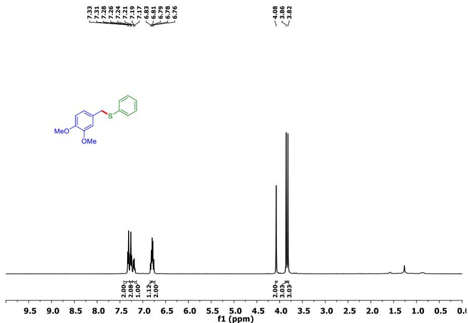
Figure 5.43.  $^1\text{H}$  NMR spectrum of (3,4-dimethoxybenzyl)(phenyl)sulfane (40a)
