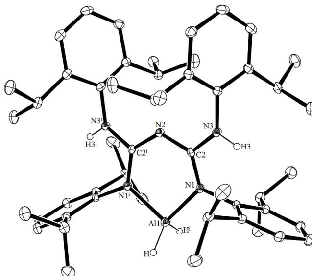
**Figure 5.8.** Molecular structure of **6**. The thermal ellipsoids are shown at 30% probability, and all the Hydrogen atoms except those bound to Nitrogen atoms are omitted for clarity. Selected bond distances (Å) and angles (deg): Al1–H 1.510(3), Al1–N1 1.8834(18), N3–H3 0.8800, N2–C2 1.344(2), N1–C2 1.341(3), N3–C2 1.364(3); N1<sup>i</sup>–Al1–N1 94.40(11), N1<sup>i</sup>–Al1–H 109.5(11), C2<sup>i</sup>–N2–C2 122.8(2), N2–C2–N1 126.6(19), N2–C2–N3 116.17(18).
