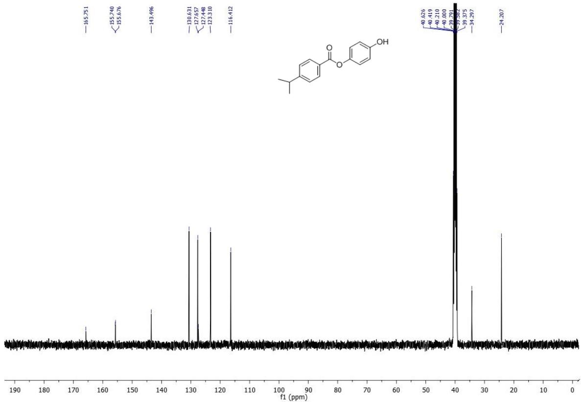
Figure 2.32. <sup>13</sup>C{<sup>1</sup>H} NMR spectrum of 4-hydroxyphenyl-4-isopropylbenzoate (3n).
