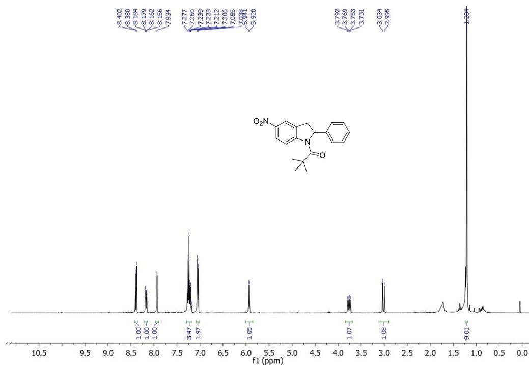
**Figure 3.19.** <sup>1</sup>H NMR spectrum of 2,2-Dimethyl-1-(5-nitro-2-phenylindolin-1-yl)propan-1-one (**2g**).
