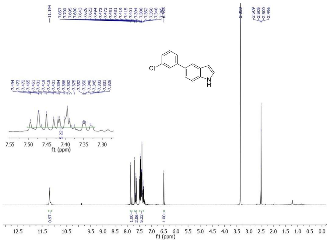
**Figure 3.65.** <sup>1</sup>H NMR spectrum of 5-(3-Chlorophenyl)-1H-indole (**1q'**).
