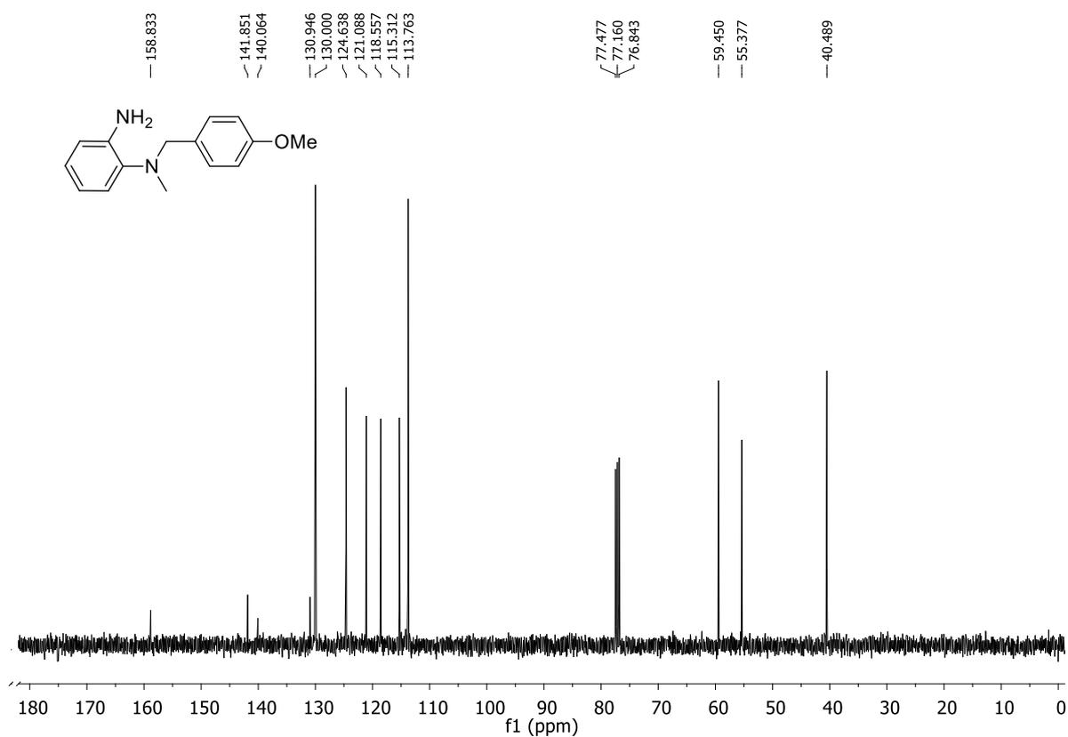
Figure 4.23. <sup>13</sup>C NMR of *N*'-(4-methoxybenzyl)-*N*'-methylbenzene-1,2-diamine (**1g**)
