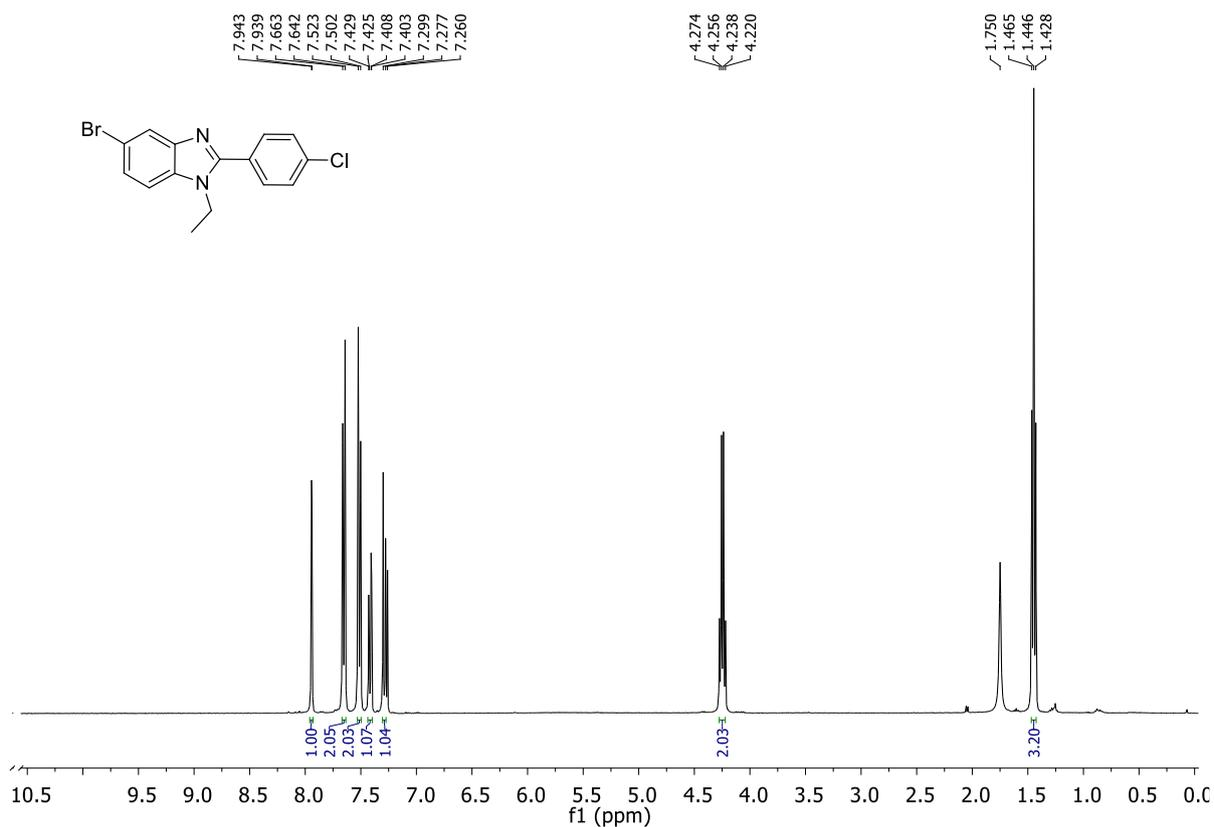
Figure 5.26 <sup>1</sup>H NMR of 5-Bromo-2-(4-chlorophenyl)-1-ethyl-benzo[d]imidazole (2k)
