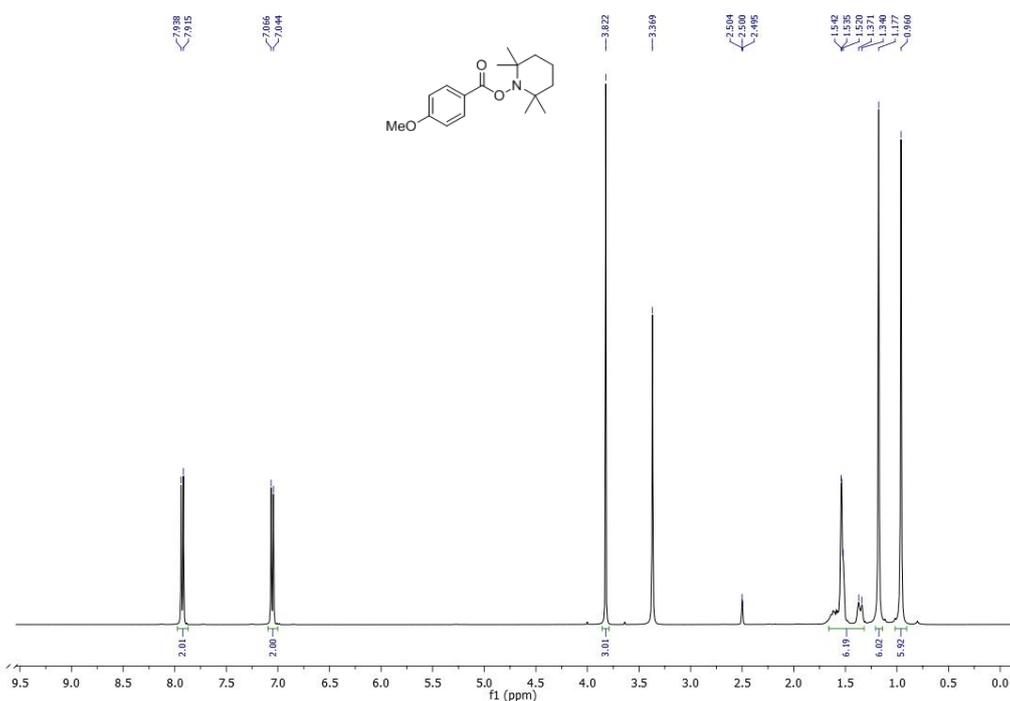
Figure 2.41.  $^1\text{H}$  NMR spectrum of 2,2,6,6-tetramethylpiperidin-1-yl-4-methoxybenzoate (**5**).
