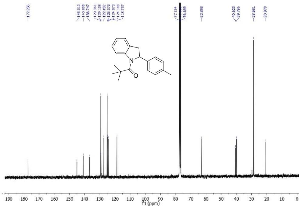
**Figure 3.82.** <sup>13</sup>C NMR spectrum of 2,2-Dimethyl-1-(2-(p-tolyl)indolin-1-yl)propan-1-one (1f).
