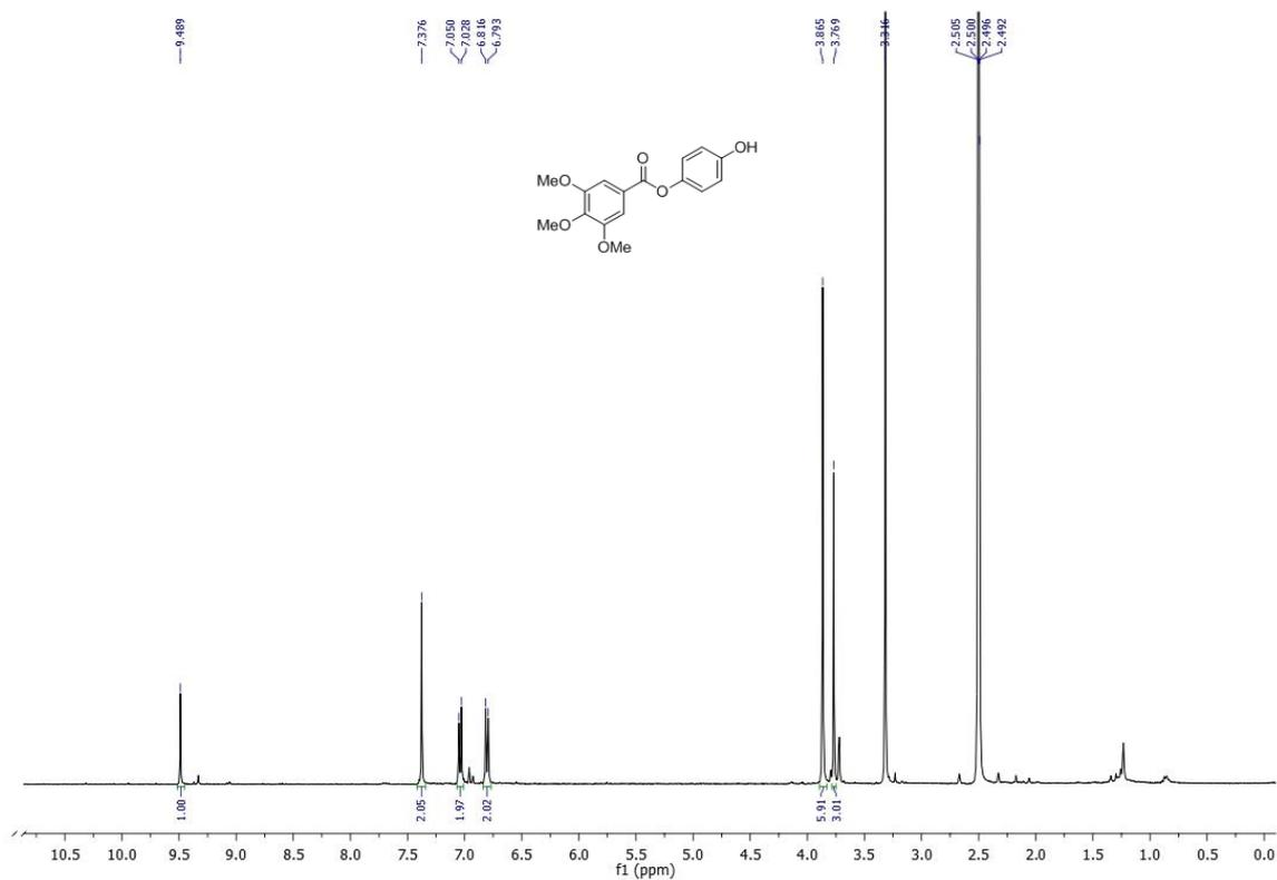
Figure 2.27.  $^1\text{H}$  NMR spectrum of 4-hydroxyphenyl-3,4,5-trimethoxybenzoate (**31**).
