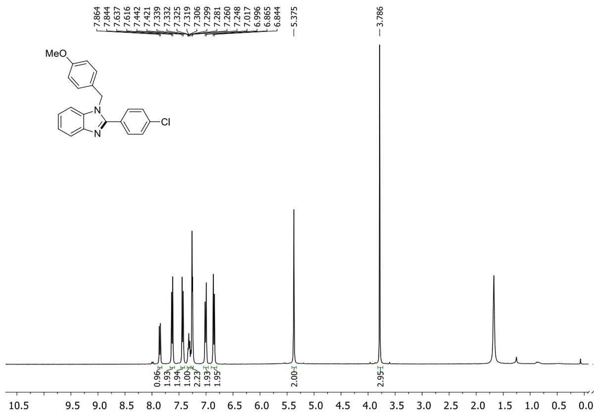
**Figure 5.38** <sup>1</sup>H NMR of 2-(4-chlorophenyl)-1-(4-methoxybenzyl)-benzo[d]imidazole (**2p'**)
