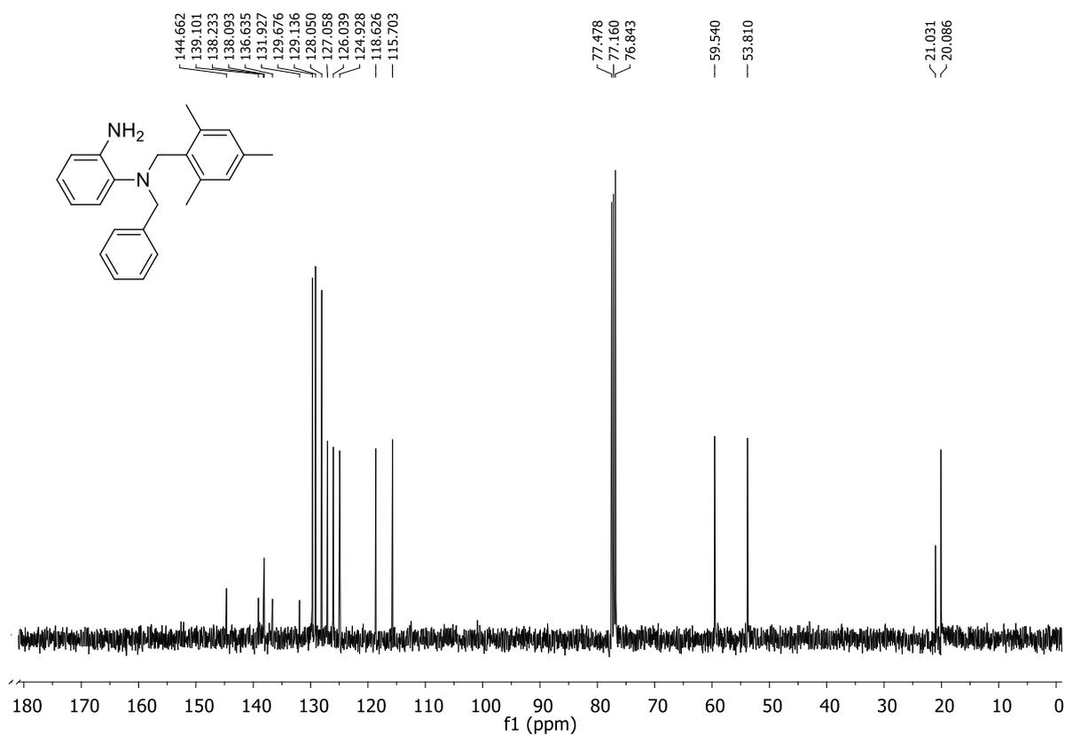
**Figure 4.47.** <sup>13</sup>C NMR of *N*<sup>1</sup>-benzyl-*N*<sup>1</sup>-(2,4,6-trimethylbenzyl)benzene-1,2-diamine (**1s**)
