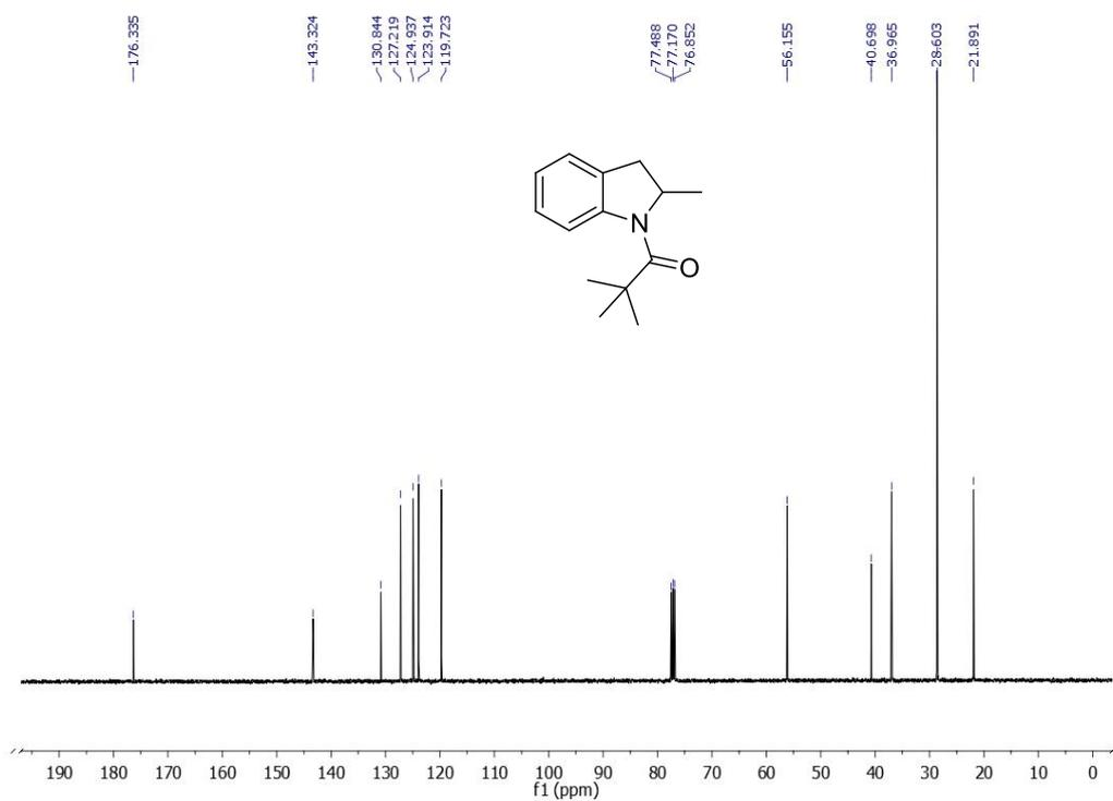
**Figure 3.80.**  $^{13}\text{C}$  NMR spectrum of 2,2-Dimethyl-1-(2-methylindolin-1-yl)propan-1-one (**1e**).
