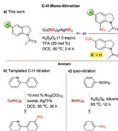
Fig. 1 C–H mono-nitration. (a) Our mono-nitration approach for non-prefunctionalized systems under mild conditions with 100% selectivity. (b) Zhang's Ru-templated *meta*-selective C–H nitration using an *ortho*-metalation template strategy.<sup>16</sup> (c) Maiti's *ipso*-nitration of aryl boronic acids.<sup>17b</sup>
