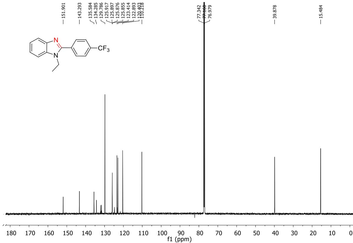
Figure 4.75. <sup>13</sup>C NMR of 1-Ethyl-2-(4-(trifluoromethyl)phenyl)-benzo[d]imidazole (2k)
