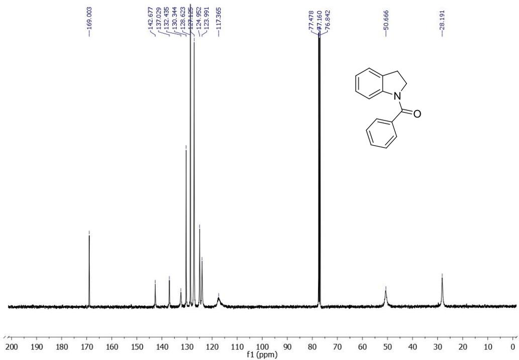
**Figure 3.90.**  $^{13}\text{C}$  NMR spectrum of Indolin-1-yl(phenyl)methanone (**1j**).
