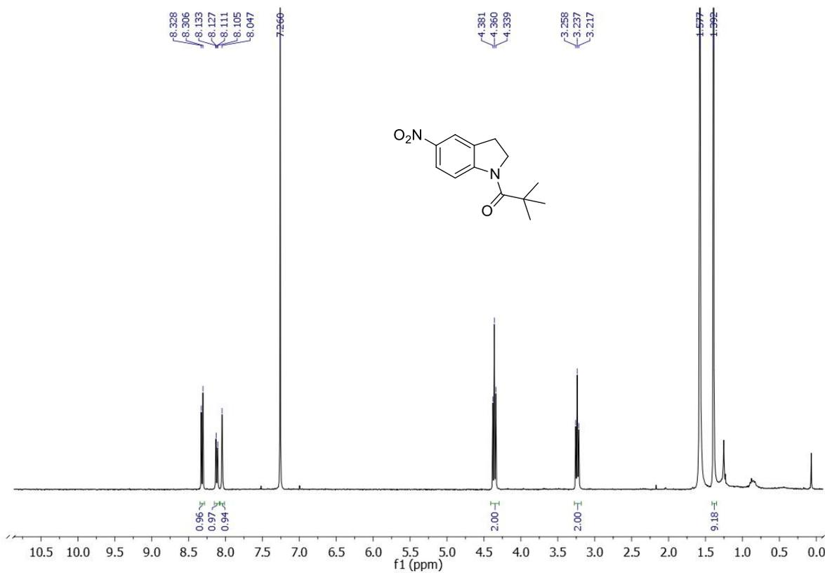
**Figure 3.21.**  $^1\text{H}$  NMR spectrum of 2,2-Dimethyl-1-(5-nitroindolin-1-yl)propan-1-one (**2h**).
