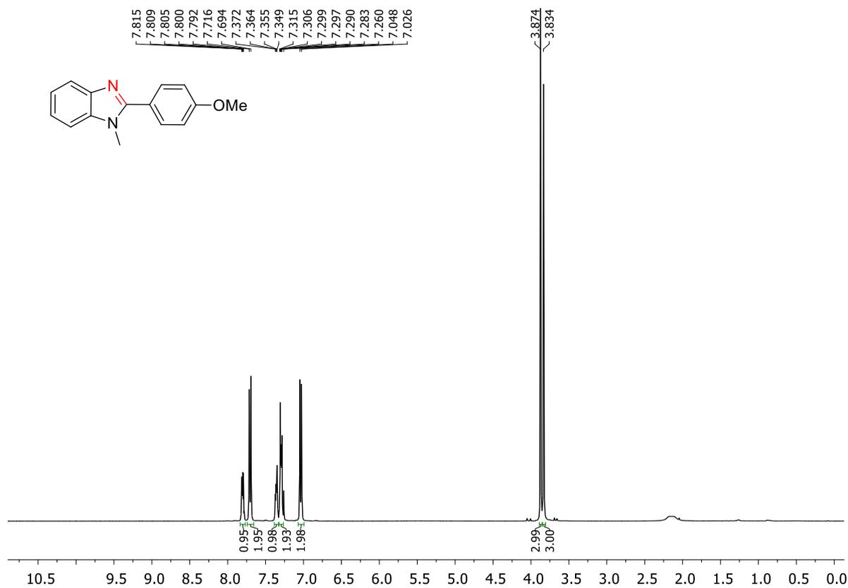
**Figure 4.66.** <sup>1</sup>H NMR of 2-(4-Methoxyphenyl)-1-methyl-benzo[d]imidazole (**2g**)
