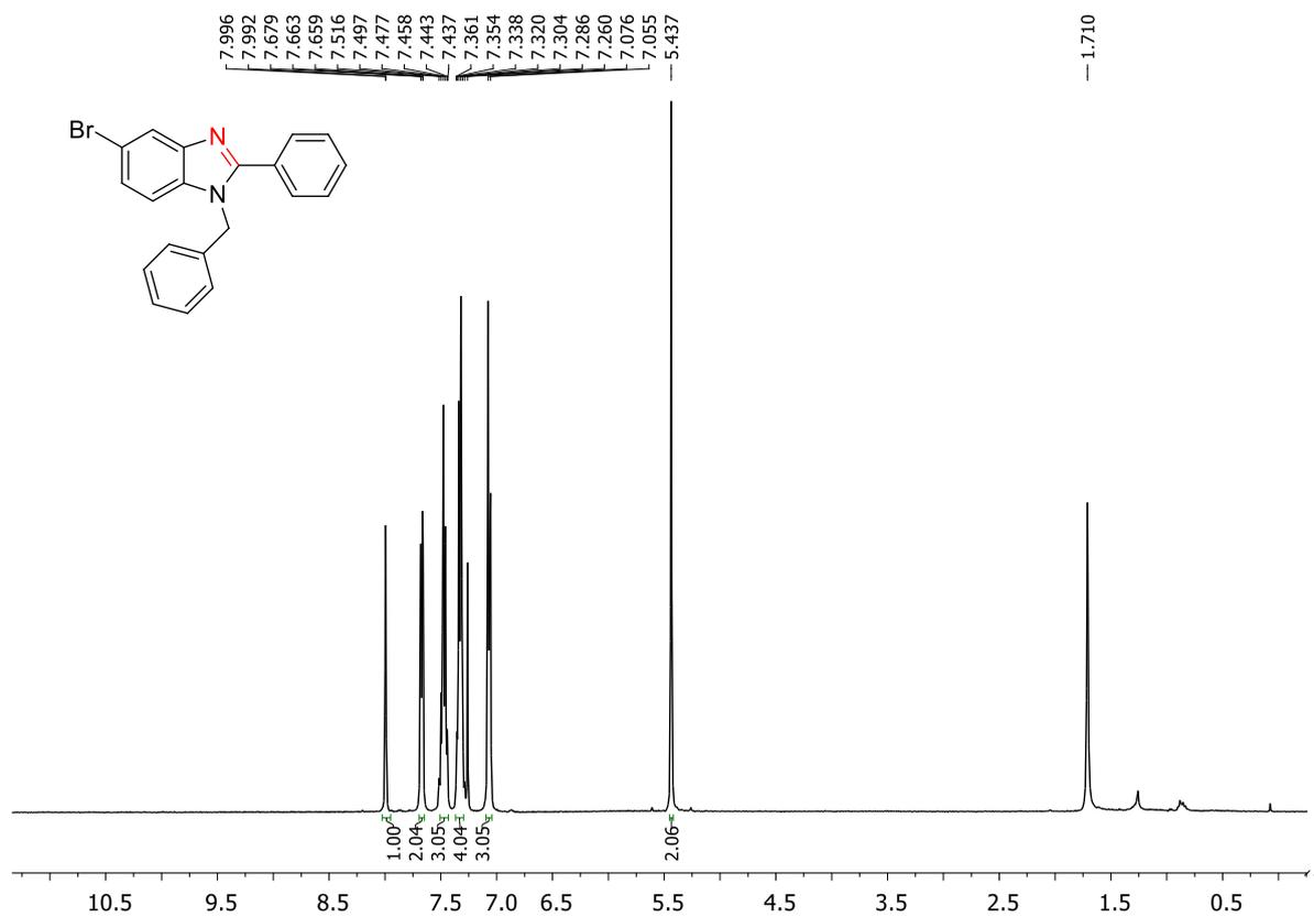
Figure 4.58.  $^1\text{H}$  NMR of 1-Benzyl-5-bromo-2-phenyl-benzo[d]imidazole (2c)
