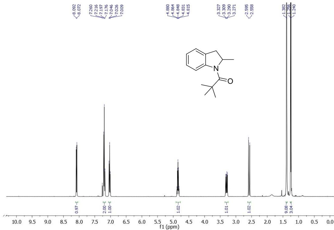
**Figure 3.79.**  $^1\text{H}$  NMR spectrum of 2,2-Dimethyl-1-(2-methylindolin-1-yl)propan-1-one (**1e**).
