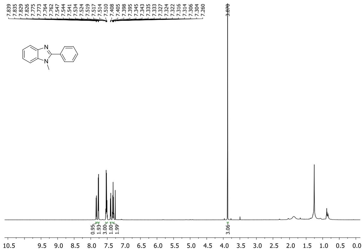
**Figure 5.14** <sup>1</sup>H NMR of 1-Methyl-2-phenyl-benzo[d]imidazole (2e)
