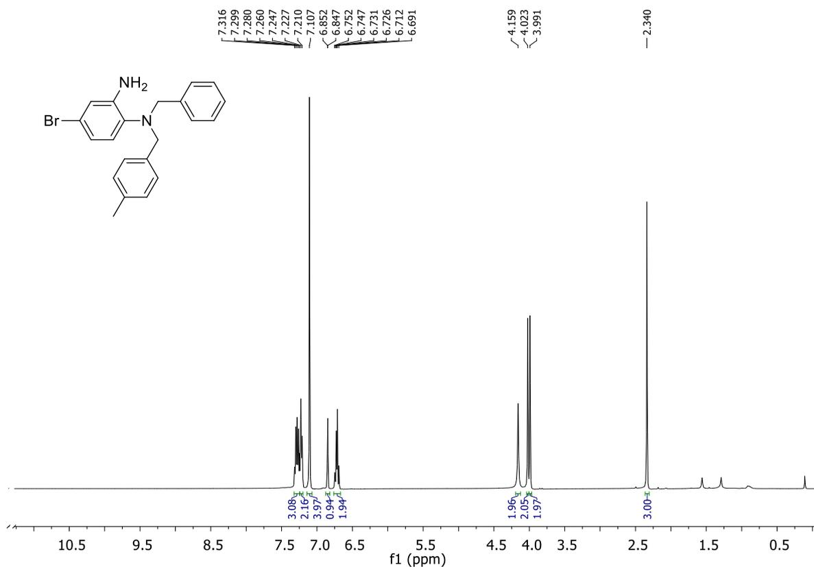
**Figure 4.38.** <sup>1</sup>H NMR of *N*<sup>1</sup>-benzyl-4-bromo-*N*<sup>1</sup>-(4-methylbenzyl)benzene-1,2-diamine (**10**)
