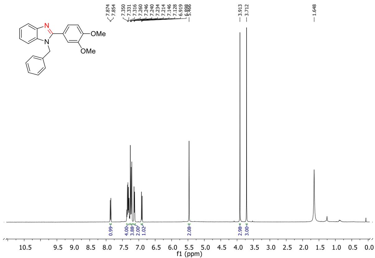
**Figure 4.88.** <sup>1</sup>H NMR of 1-Benzyl-2-(3,4-dimethoxyphenyl)-benzo[d]imidazole (**2r**)
