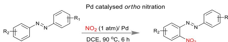
**Scheme 3.3.** Sun's Pd catalysed *ortho* nitration approach.
