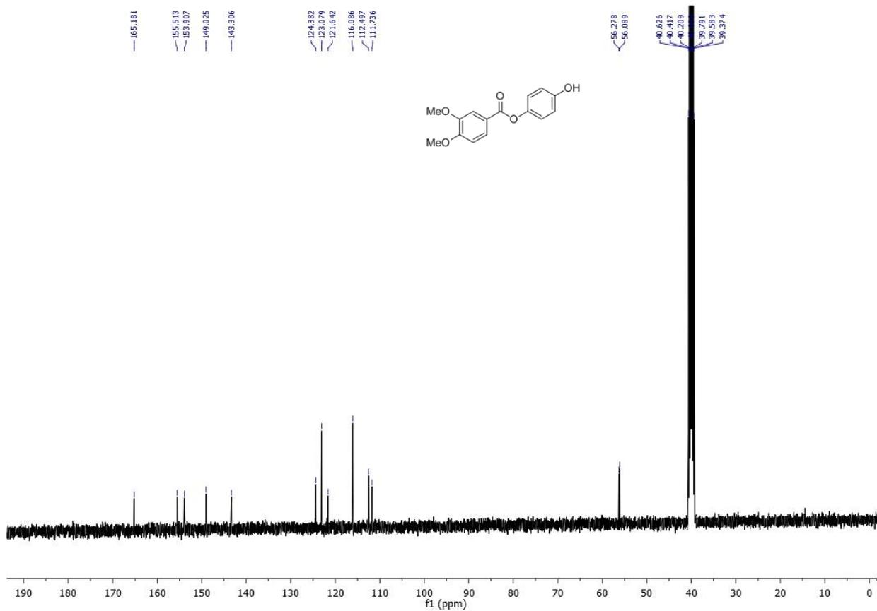
Figure 2.26.  $^{13}\text{C}\{^1\text{H}\}$  NMR spectrum of 4-hydroxyphenyl-3,4-dimethoxybenzoate (**3k**).
