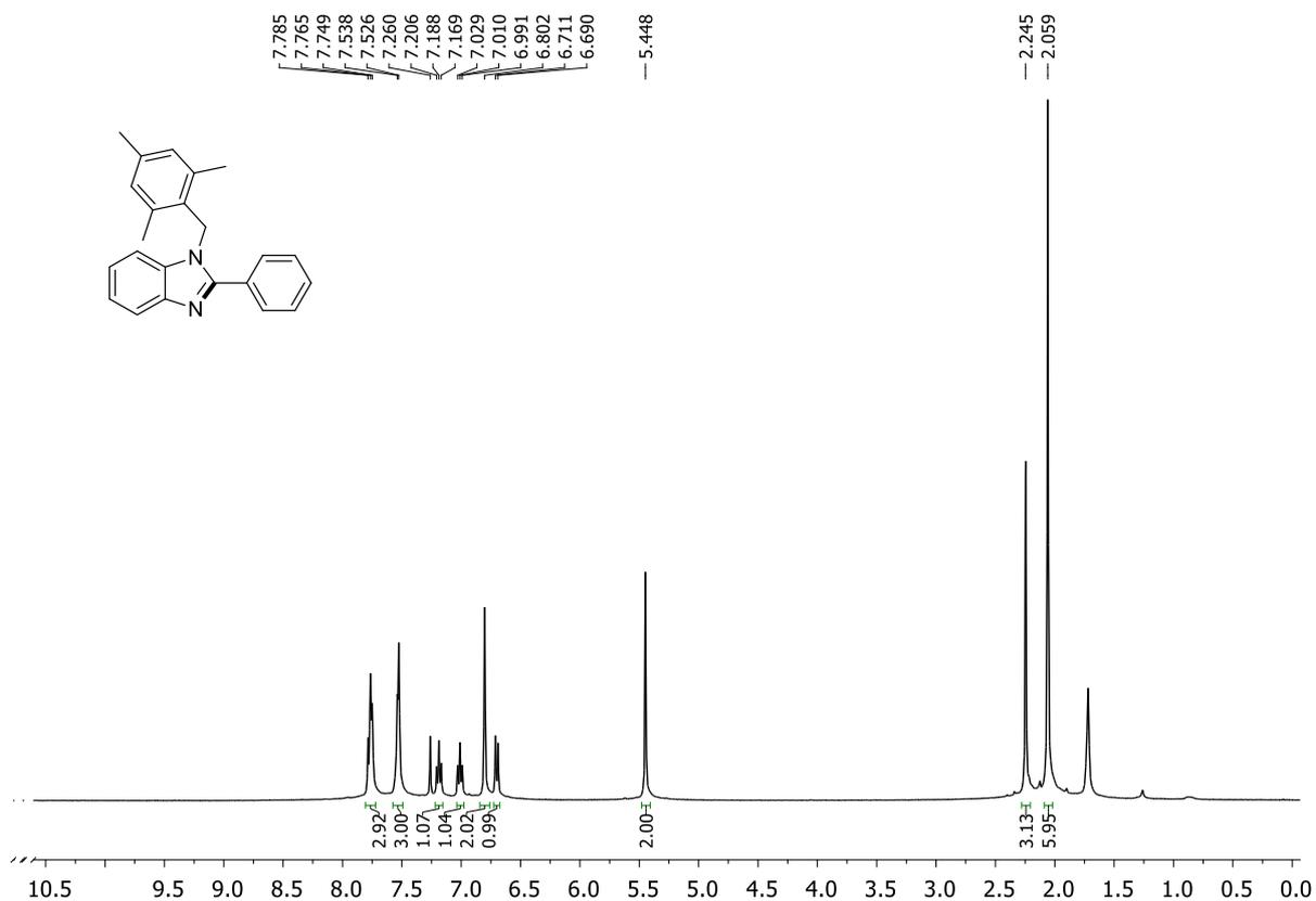
Figure 5.42 <sup>1</sup>H NMR of 2-Phenyl-1-(2,4,6-trimethylbenzyl)-benzo[d]imidazole (2q')
