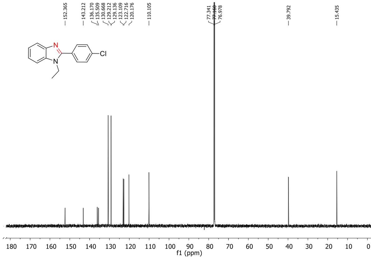
Figure 4.73. <sup>13</sup>C NMR of 2-(4-Chlorophenyl)-1-ethyl-benzo[d]imidazole (2j)
