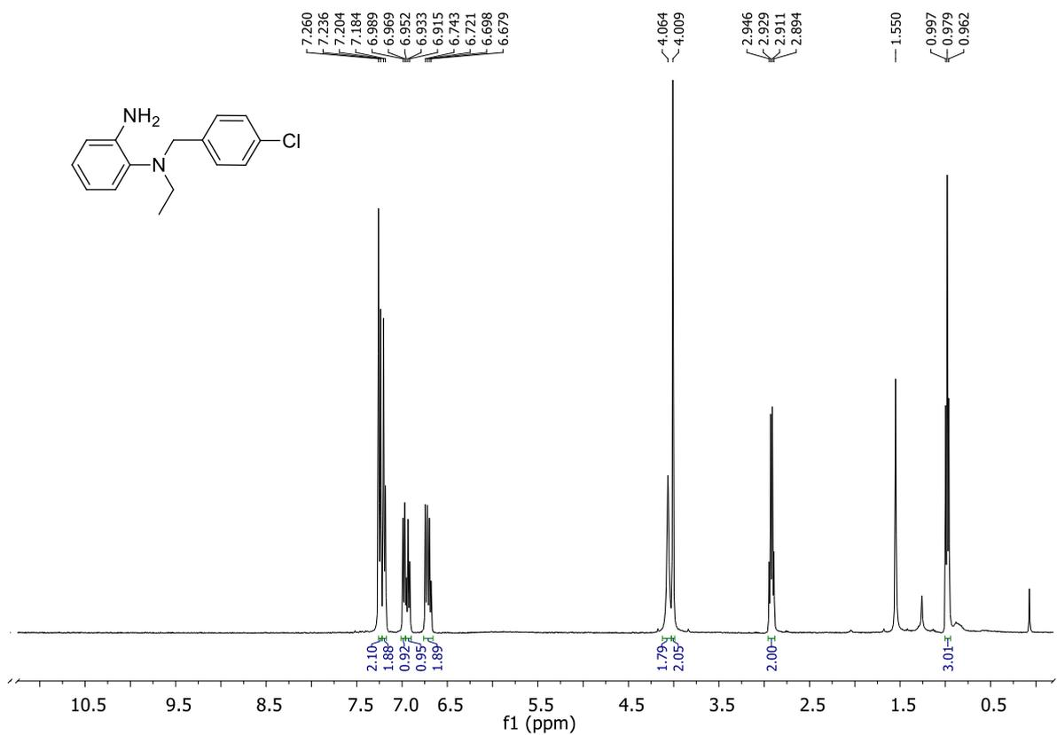
Figure 4.28. <sup>1</sup>H NMR of *N*<sup>1</sup>-(4-chlorobenzyl)-*N*<sup>1</sup>-ethylbenzene-1,2-diamine (**1j**)
