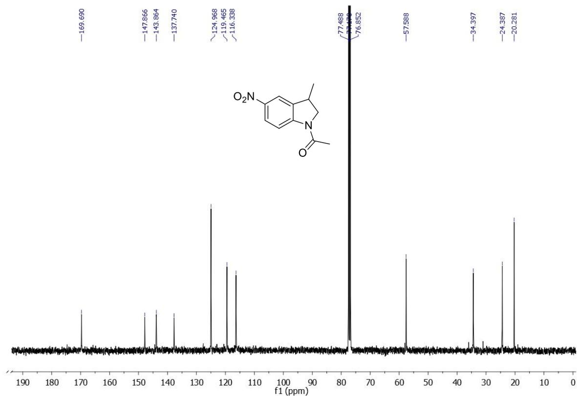
**Figure 3.10.** <sup>13</sup>C NMR spectrum of 1-(3-Methyl-5-nitroindolin-1-yl)ethanone (**2b**).
