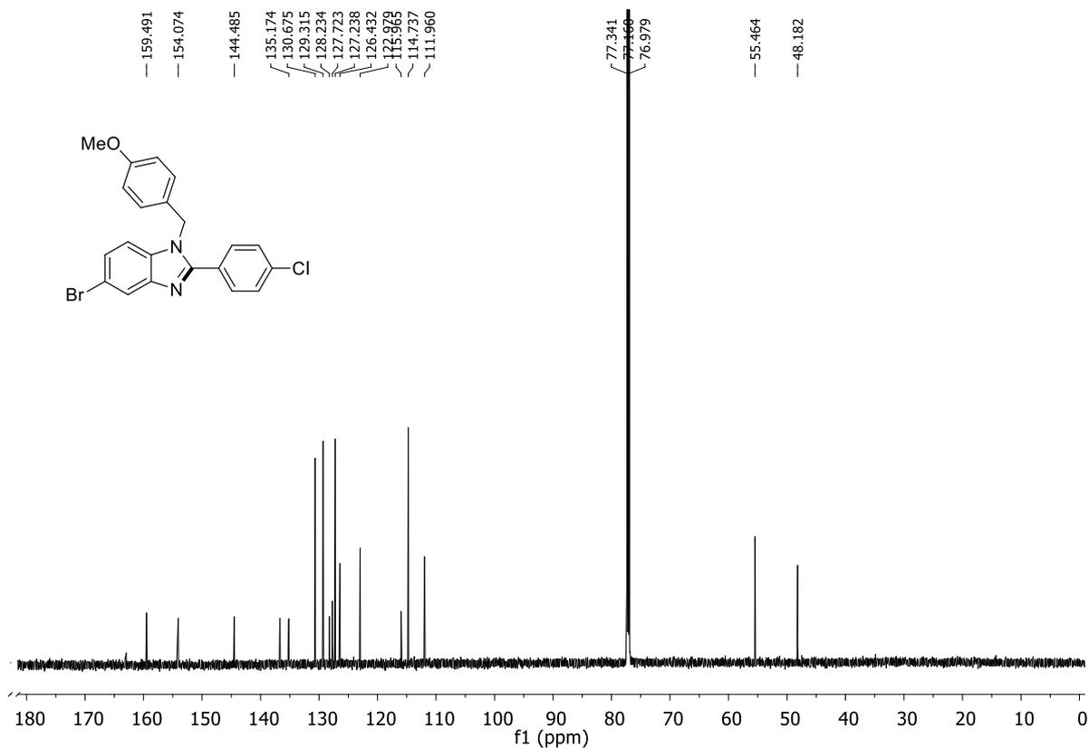
**Figure 5.47** <sup>13</sup>C NMR of 5-Bromo-2-(4-chlorophenyl)-1-(4-methoxybenzyl)-benzo[d]imidazole (**2r'**)
