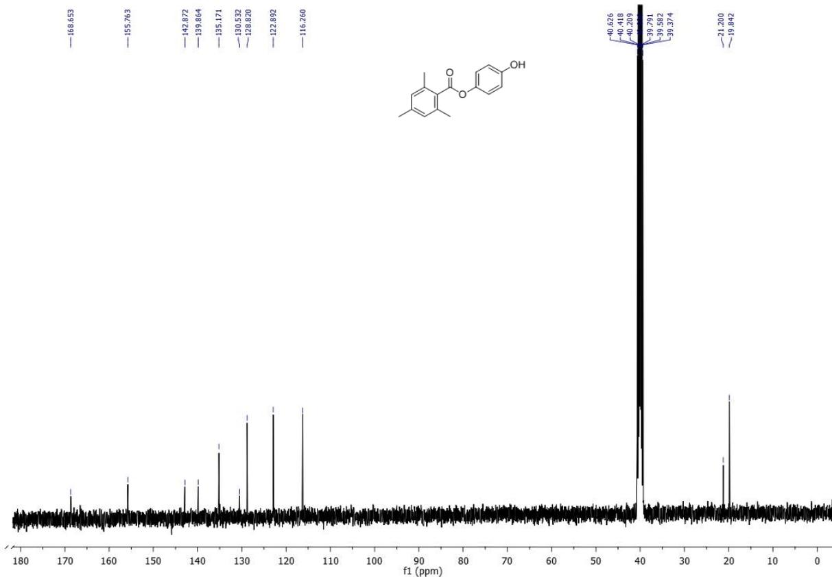
**Figure 2.30.**  $^{13}\text{C}\{^1\text{H}\}$  NMR spectrum of 4-hydroxyphenyl-2,4,6-trimethylbenzoate (**3m**).
