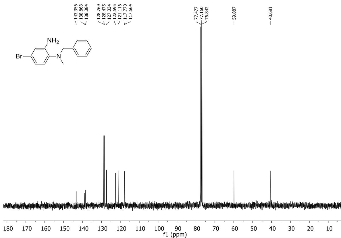
Figure 4.21. <sup>13</sup>C NMR of *N*<sup>1</sup>-Benzyl-4-bromo-*N*<sup>1</sup>-methylbenzene-1,2-diamine (**1f**)
