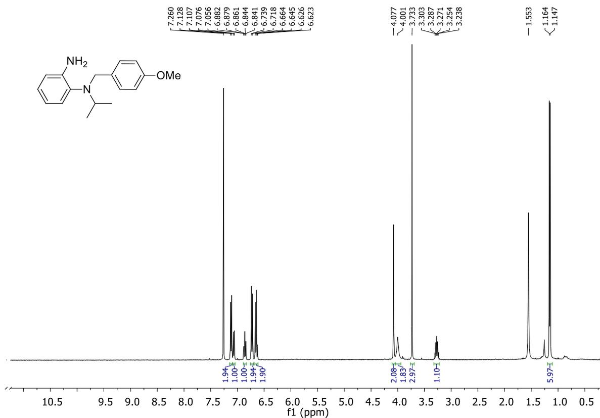
**Figure 4.32.** <sup>1</sup>H NMR of *N*<sup>1</sup>-isopropyl-*N*<sup>1</sup>-(4-methoxybenzyl)benzene-1,2-diamine (**11**)
