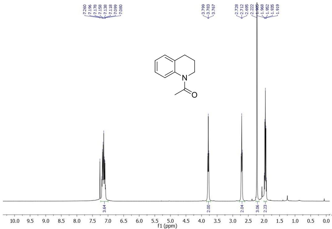
**Figure 3.107.** <sup>1</sup>H NMR spectrum of 1-(3,4-Dihydroquinolin-1(2H)-yl)ethanone (4).
