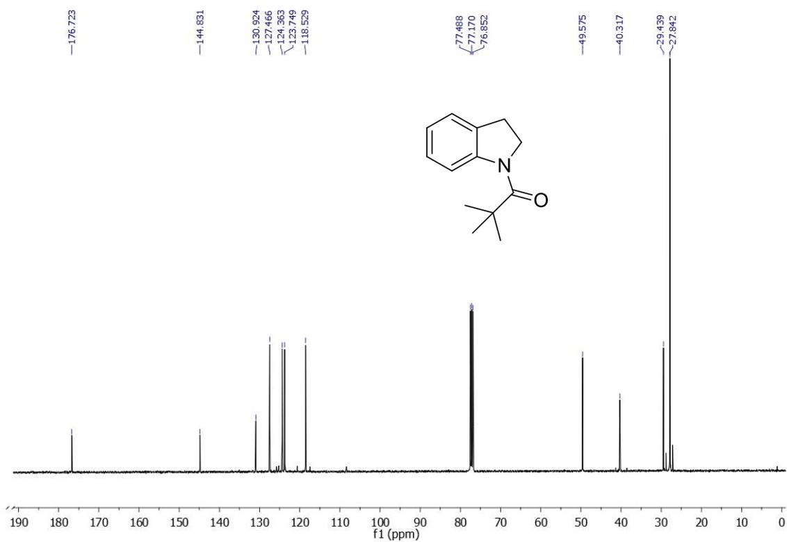
**Figure 3.86.** <sup>13</sup>C NMR spectrum of 1-(Indolin-1-yl)-2,2-dimethylpropan-1-one (**1h**).
