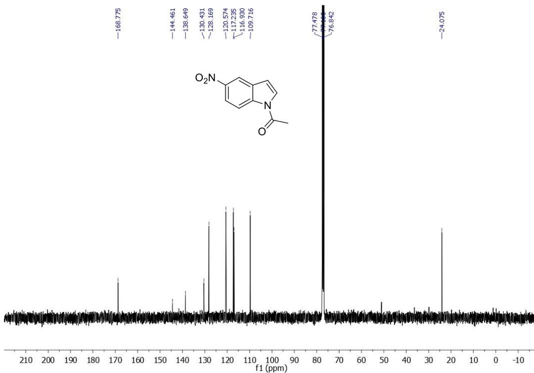
**Figure 3.46.**  $^{13}\text{C}$  NMR spectrum of 1-(5-Nitro-1H-indol-1-yl)ethanone (**3a**).
