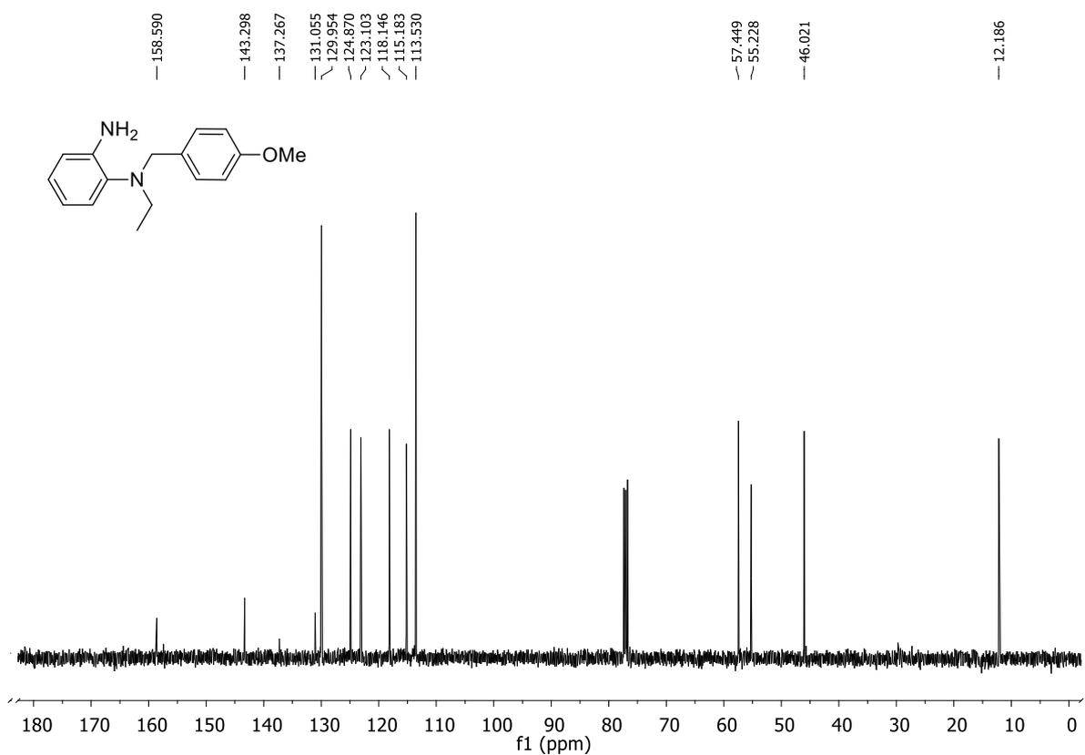
**Figure 4.25.** <sup>13</sup>C NMR of *N*<sup>1</sup>-ethyl-*N*<sup>1</sup>-(4-methoxybenzyl)benzene-1,2-diamine (**1h**)
