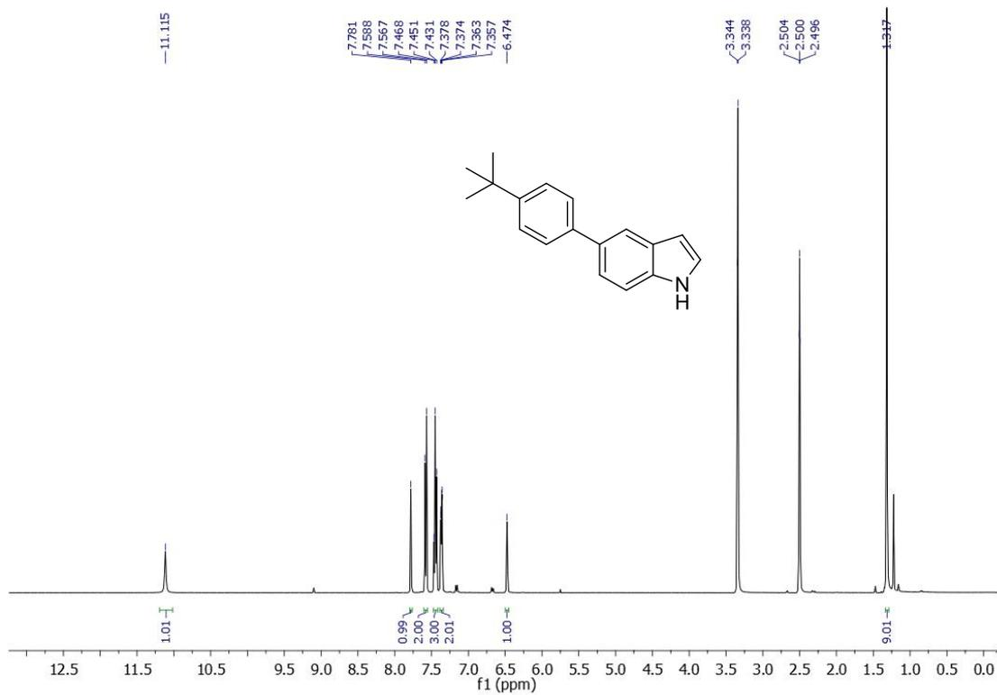
**Figure 3.61.** <sup>1</sup>H NMR spectrum of 5-(4-(tert-Butyl)phenyl)-1H-indole (**1o'**).
