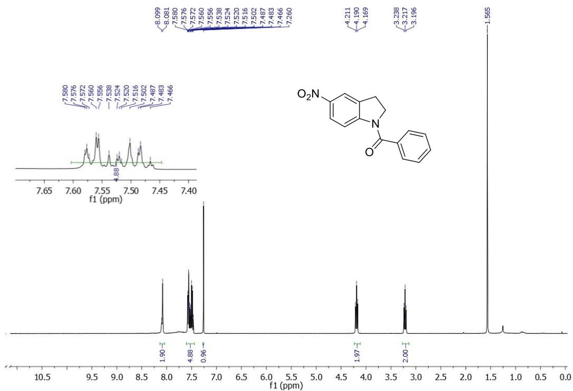
**Figure 3.25.** <sup>1</sup>H NMR spectrum of (5-Nitroindolin-1-yl)(phenyl)methanone (**2j**).
