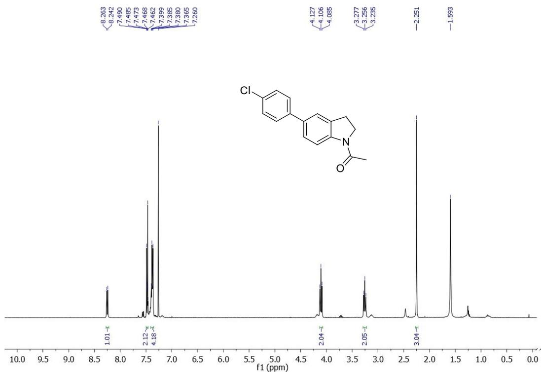
**Figure 3.105.** <sup>1</sup>H NMR spectrum of 1-(5-(4-Chlorophenyl)indolin-1-yl)ethanone (1s).
