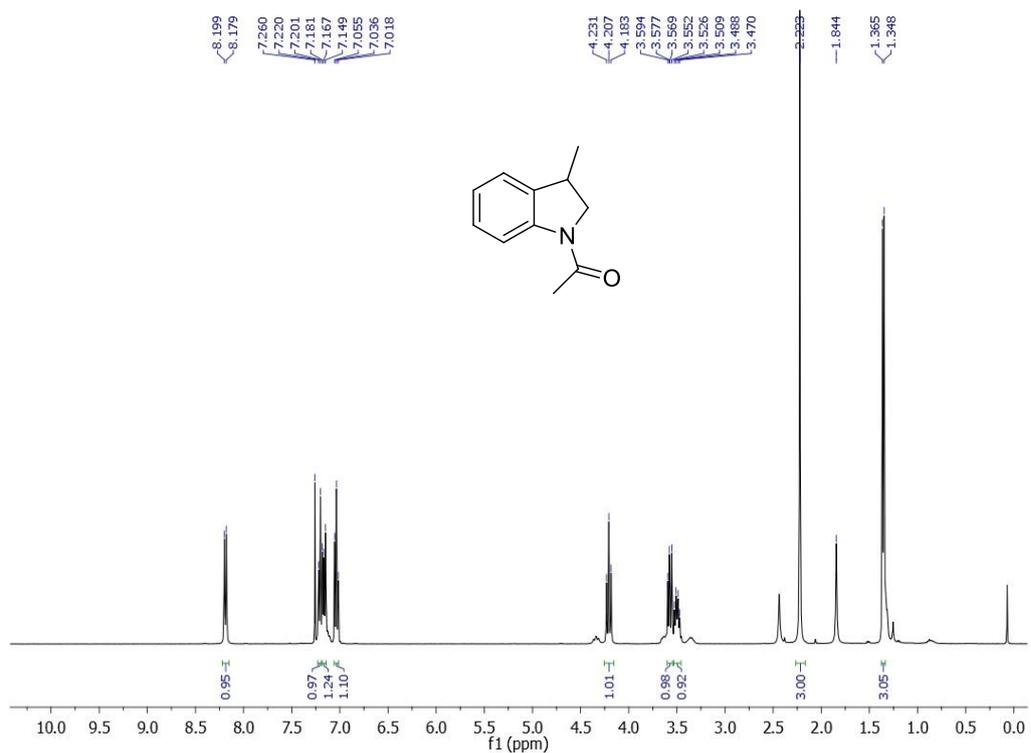
**Figure 3.73.**  $^1\text{H}$  NMR spectrum of 1-(3-Methylindolin-1-yl)ethanone (**1b**).
