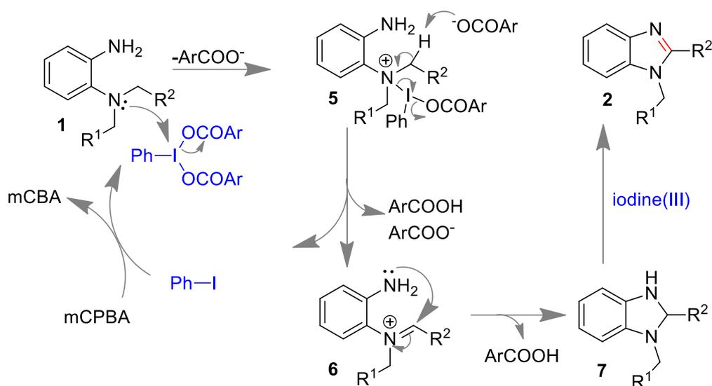
**Figure 4.6** Plausible mechanism of the reaction.
