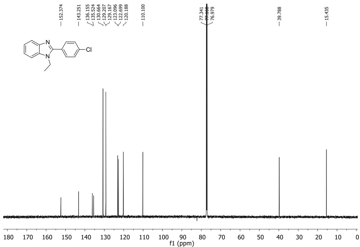
Figure 5.25 <sup>13</sup>C NMR of 2-(4-Chlorophenyl)-1-ethyl-benzo[d]imidazole (2j)
