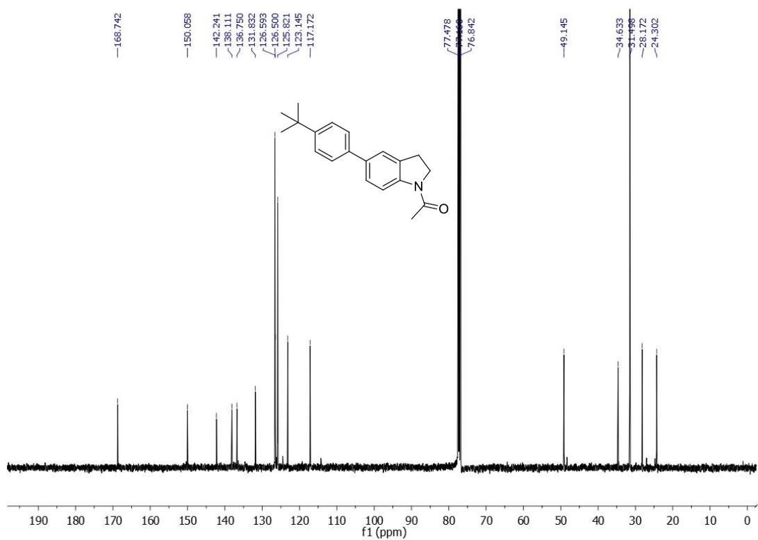
**Figure 3.98.** <sup>13</sup>C NMR spectrum of 1-(5-(4-(tert-Butyl)phenyl)indolin-1-yl)ethanone (**10**).
