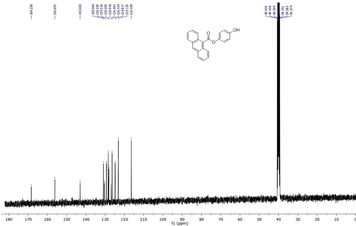
Figure 2.38.  $^{13}\text{C}\{^1\text{H}\}$  NMR spectrum of 4-hydroxyphenyl-anthracene-9-carboxylate (3q).
