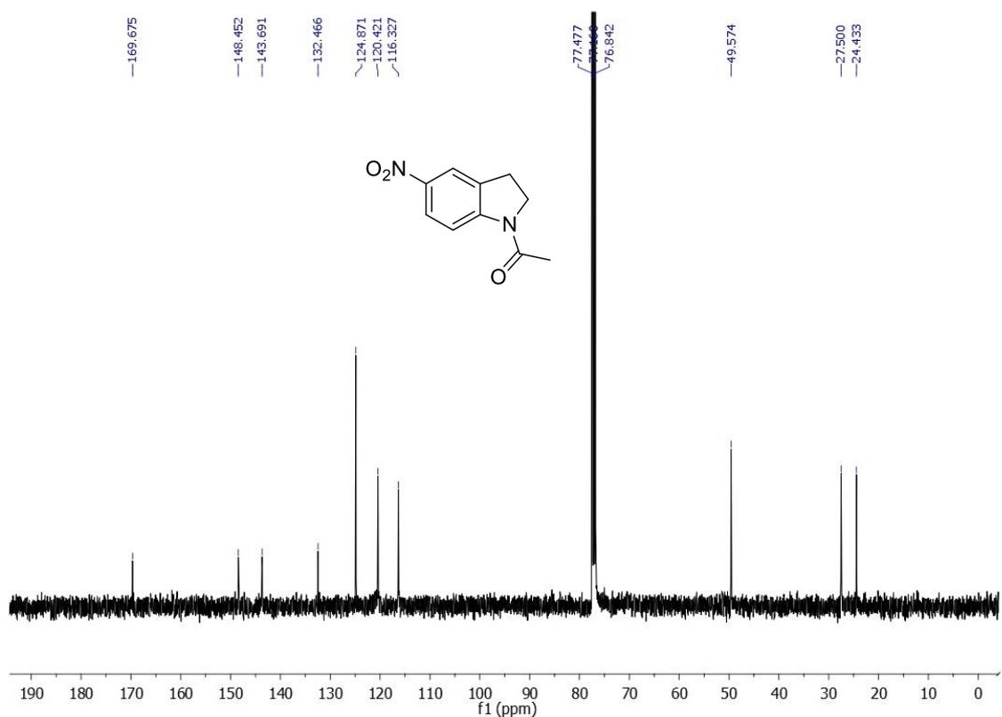
**Figure 3.8.**  $^{13}\text{C}$  NMR spectrum of 1-(5-Nitroindolin-1-yl)ethanone (**2a**).
