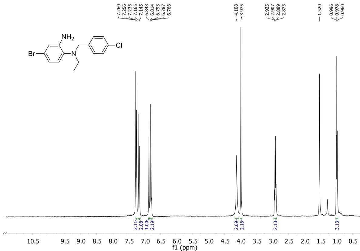
Figure 4.34. <sup>1</sup>H NMR of 4-Bromo-*N*'-(4-chlorobenzyl)-*N*'-ethylbenzene-1,2-diamine (**1m**)
