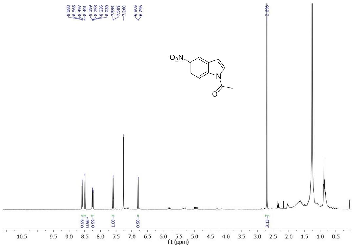
**Figure 3.45.**  $^1\text{H}$  NMR spectrum of 1-(5-Nitro-1H-indol-1-yl)ethanone (**3a**).
