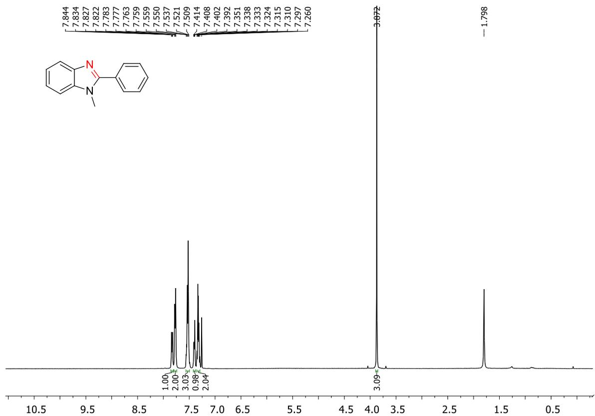
**Figure 4.62.** <sup>1</sup>H NMR of 1-Methyl-2-phenyl-benzo[d]imidazole (**2e**)
