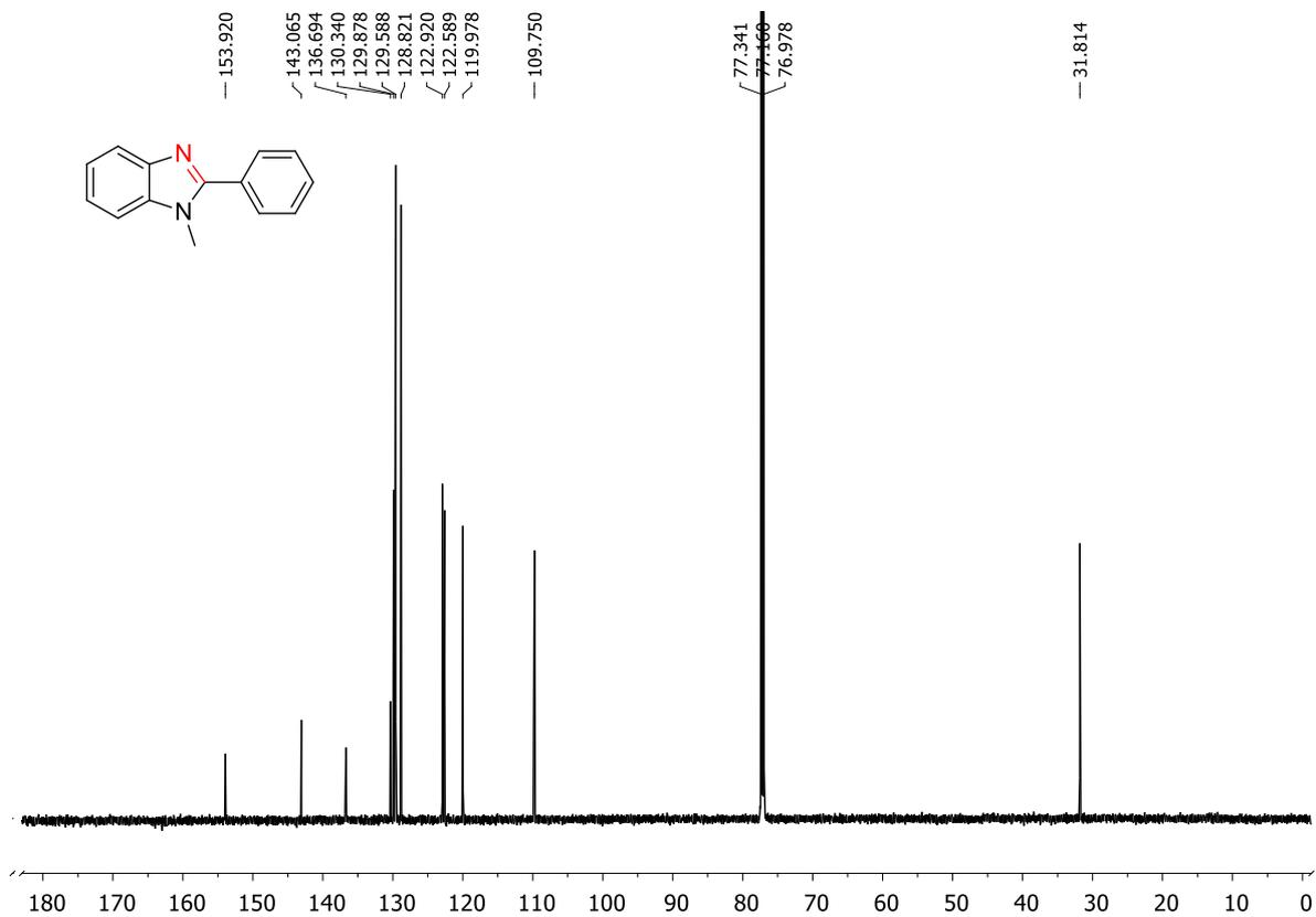
**Figure 4.63.** <sup>13</sup>C NMR of 1-Methyl-2-phenyl-benzo[d]imidazole (**2e**)
