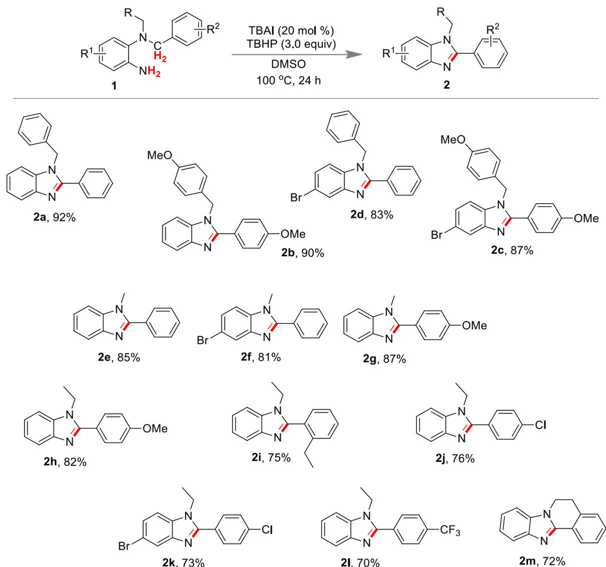
**Figure 5.2** Substrate scope for C(sp<sup>3</sup>)-H imination reaction.
