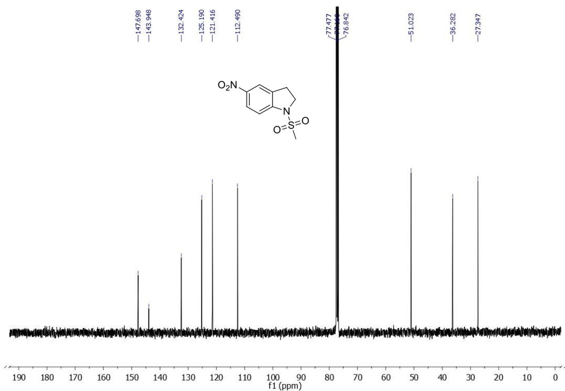
**Figure 3.14.** <sup>13</sup>C NMR spectrum of 1-(Methylsulfonyl)-5-nitroindoline (**2d**).
