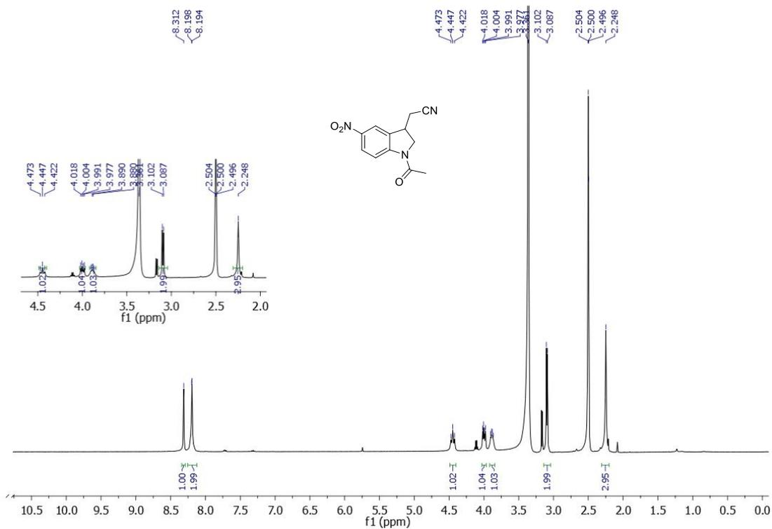
**Figure 3.11.** <sup>1</sup>H NMR spectrum of 2-(1-Acetyl-5-nitroindolin-3-yl)acetonitrile (**2c**).
