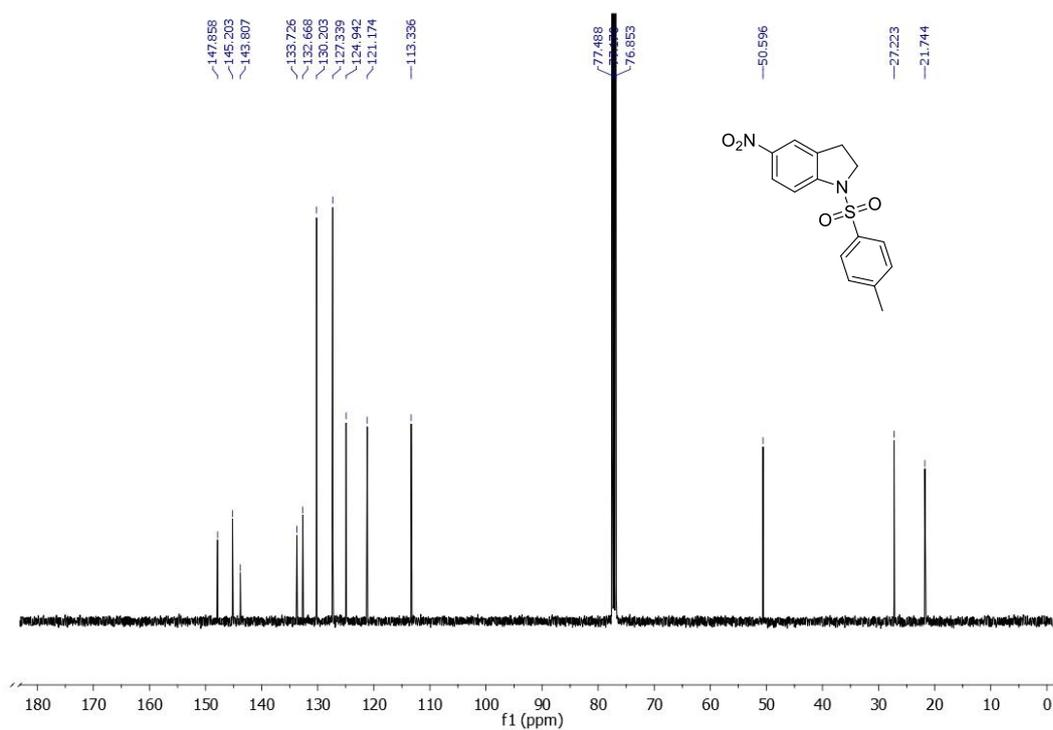
**Figure 3.24.** <sup>13</sup>C NMR spectrum of 5-Nitro-1-tosylindoline (**2i**).
