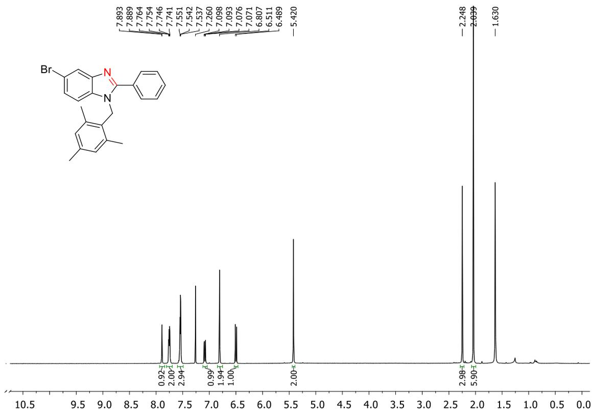
**Figure 4.98.** <sup>1</sup>H NMR of 5-Bromo-2-phenyl-1-(2,4,6-trimethylbenzyl)-benzo[d]imidazole (2t')
