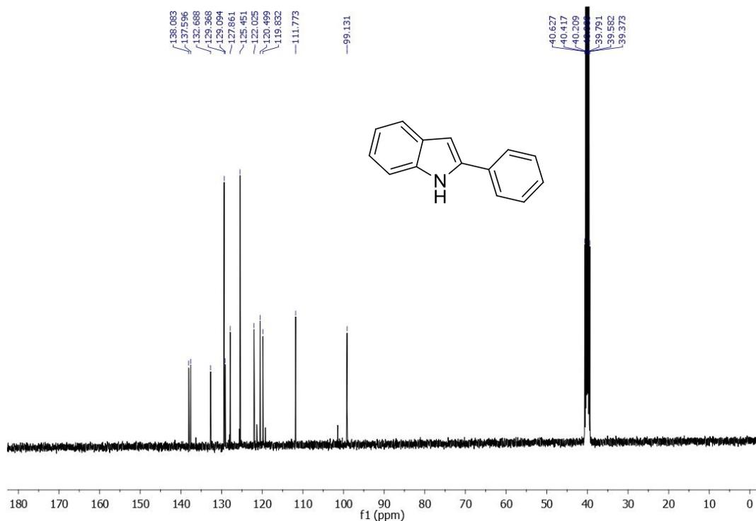
Figure 3.56.  $^{13}\text{C}$  NMR spectrum of 2-Phenyl-1H-indole (**1g'**).
