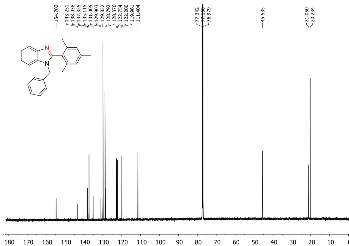
Figure 4.93.  $^{13}\text{C}$  NMR of 1-Benzyl-2-mesityl-benzo[d]imidazole (**2s**)
