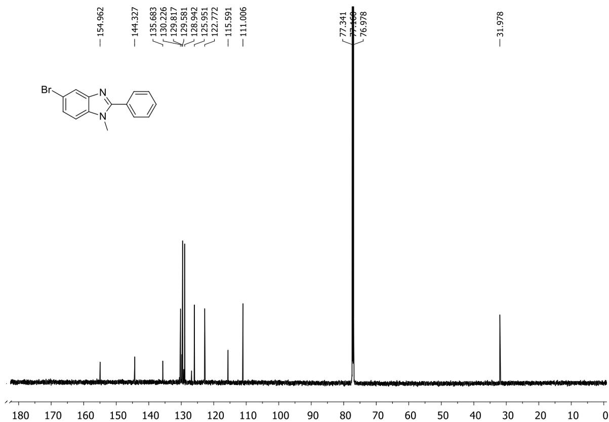
**Figure 5.17** <sup>13</sup>C NMR of 5-Bromo-1-methyl-2-phenyl-benzo[d]imidazole (**2f**)
