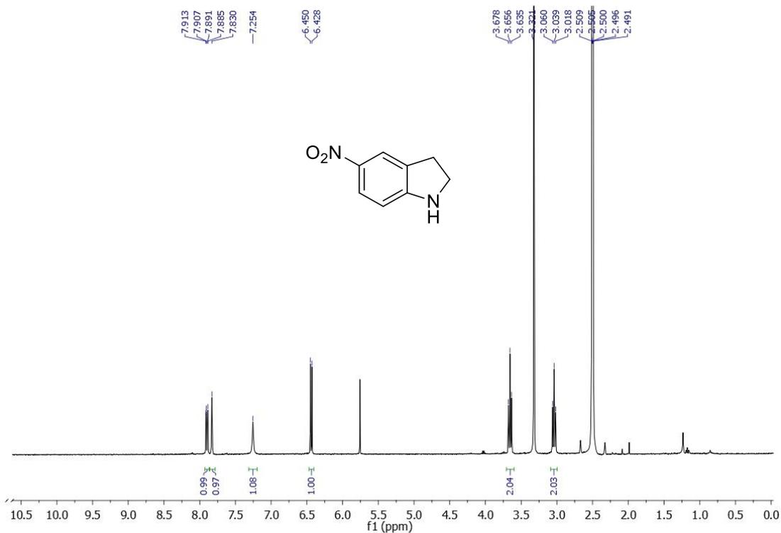
**Figure 3.49.**  $^1\text{H}$  NMR spectrum of 5-Nitroindoline (**3c**).
