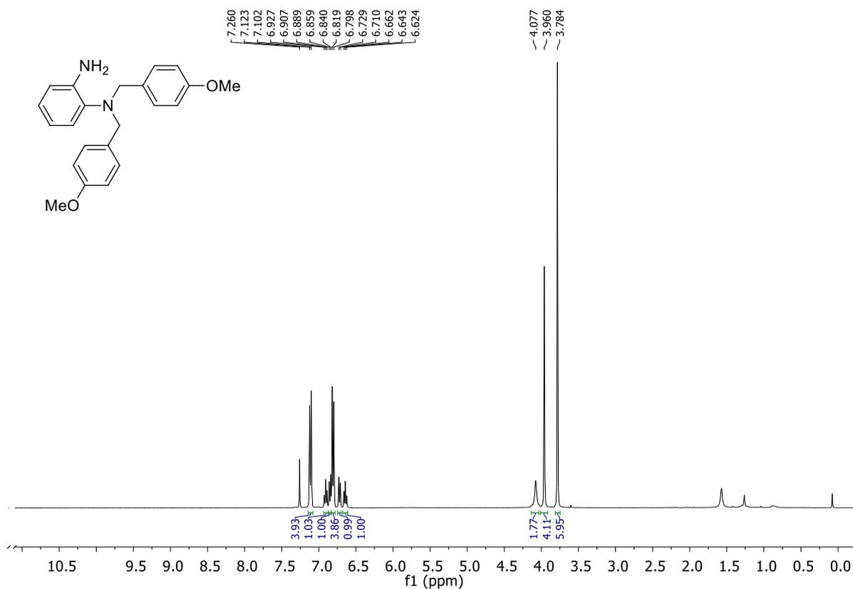
Figure 4.12. <sup>1</sup>H NMR of *N,N'*- bis(4-methoxybenzyl)benzene-1,2-diamine (**1b**)
