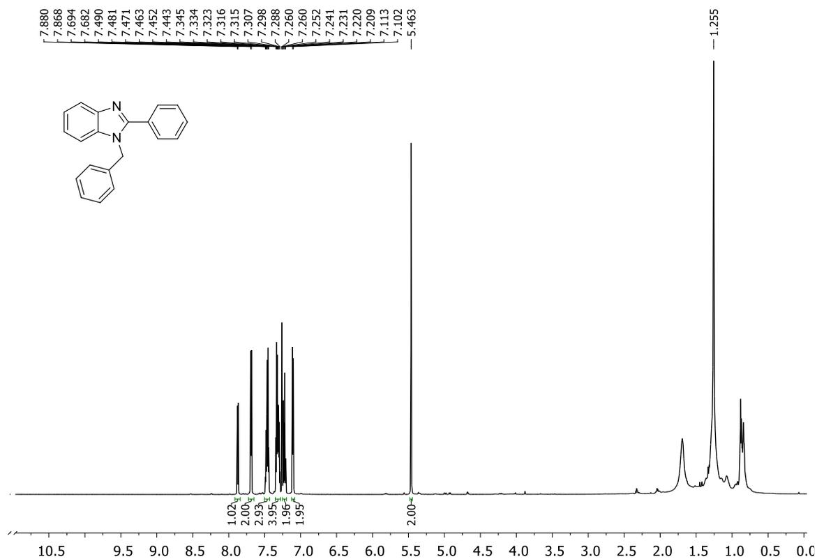
**Figure 5.6**  $^1\text{H}$  NMR of 1-Benzyl-2-phenyl-benzo[d]imidazole (**2a**)
