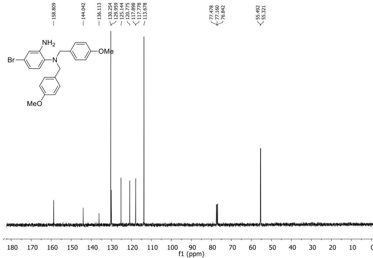
**Figure 4.17.** <sup>13</sup>C NMR of 4-Bromo-*N,N'*-bis(4-methoxybenzyl)benzene-1,2-diamine (**1d**)
