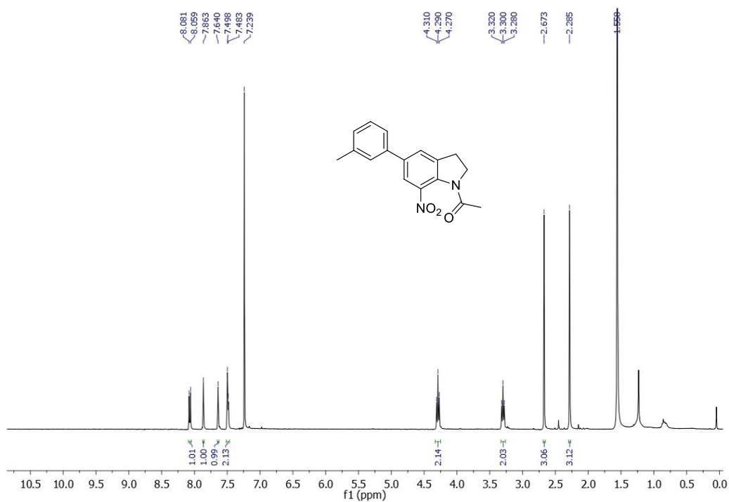
**Figure 3.31.** <sup>1</sup>H NMR spectrum of 1-(7-Nitro-5-(m-tolyl)indolin-1-yl)ethanone (**2m**).
