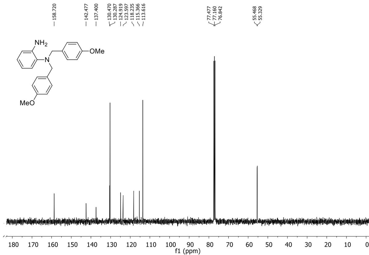
Figure 4.13. <sup>13</sup>C NMR of *N,N'*- bis(4-methoxybenzyl)benzene-1,2-diamine (**1b**)
