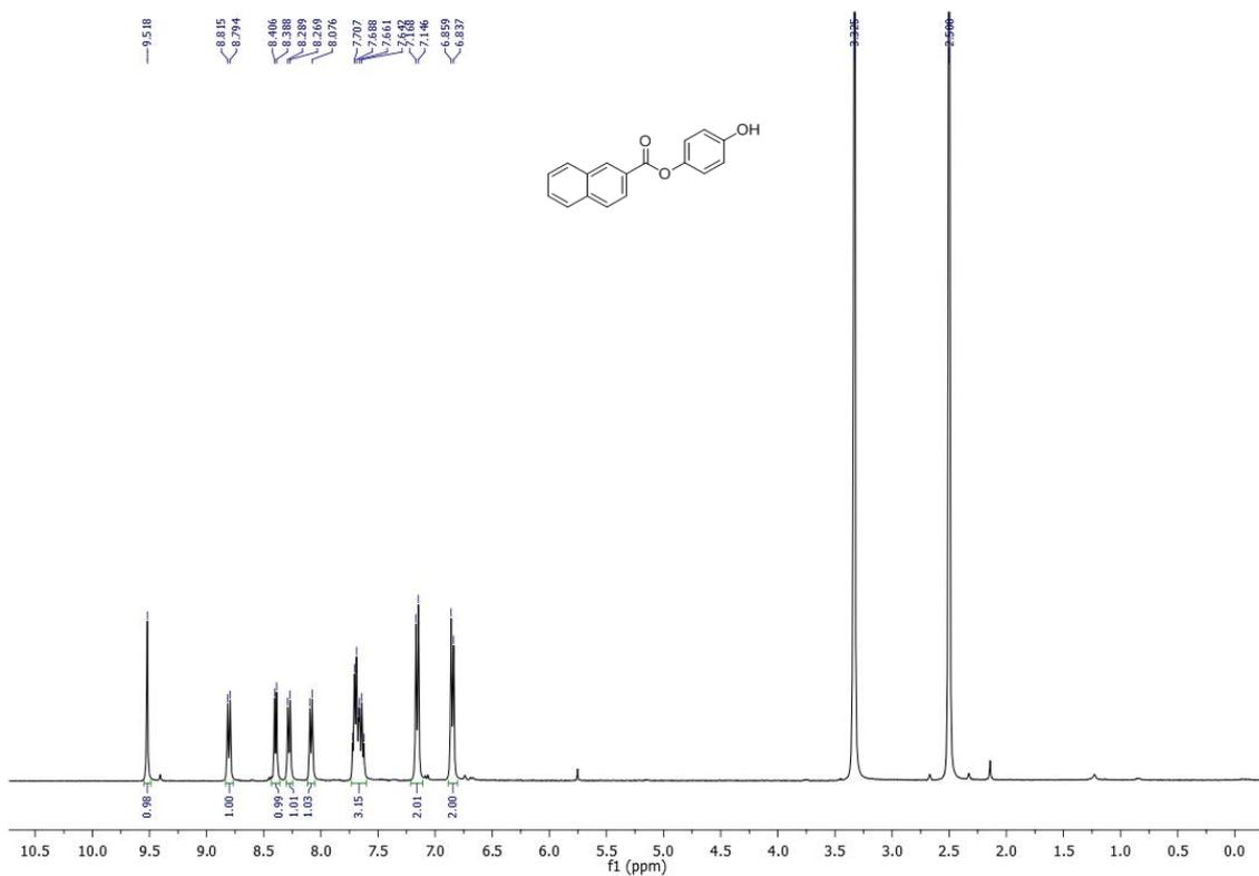
**Figure 2.35.**  $^1\text{H}$  NMR spectrum of 4-hydroxyphenyl-2-naphthoate (**3p**).
