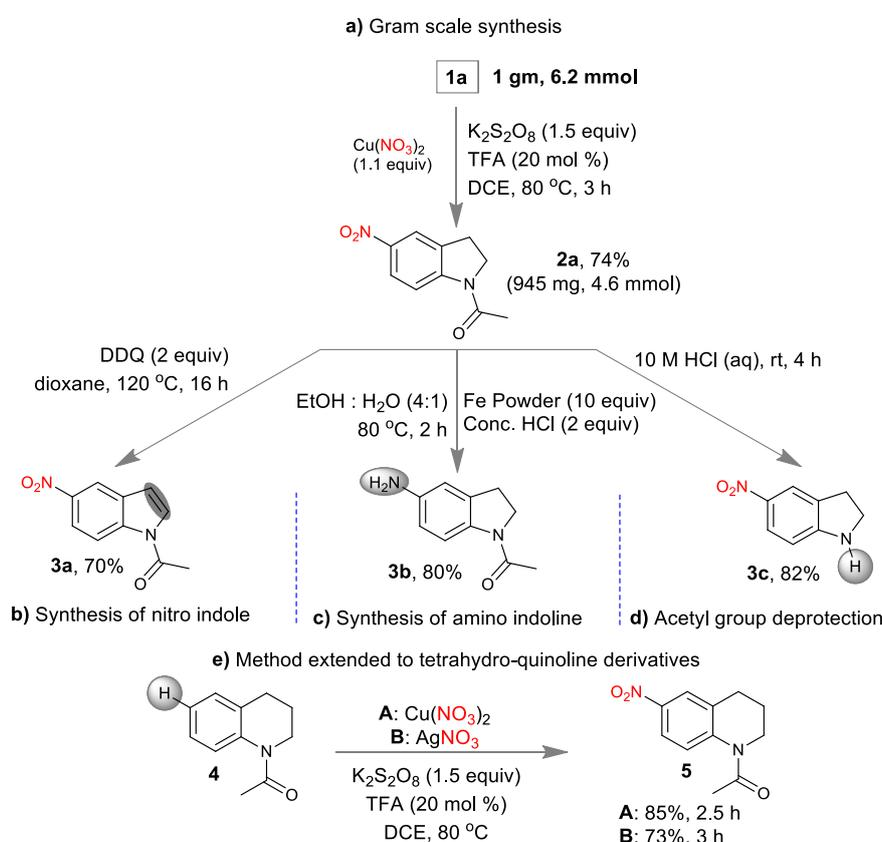
**Figure 3.6.** Post synthetic application. a) Gram scale synthesis of **2a**. b) Oxidation of nitroindoline to nitroindole. c) Reduction of nitro-indoline to amino-indoline. d) Acetyl group deprotection. e) Nitration of tetrahydroquinoline derivatives.
