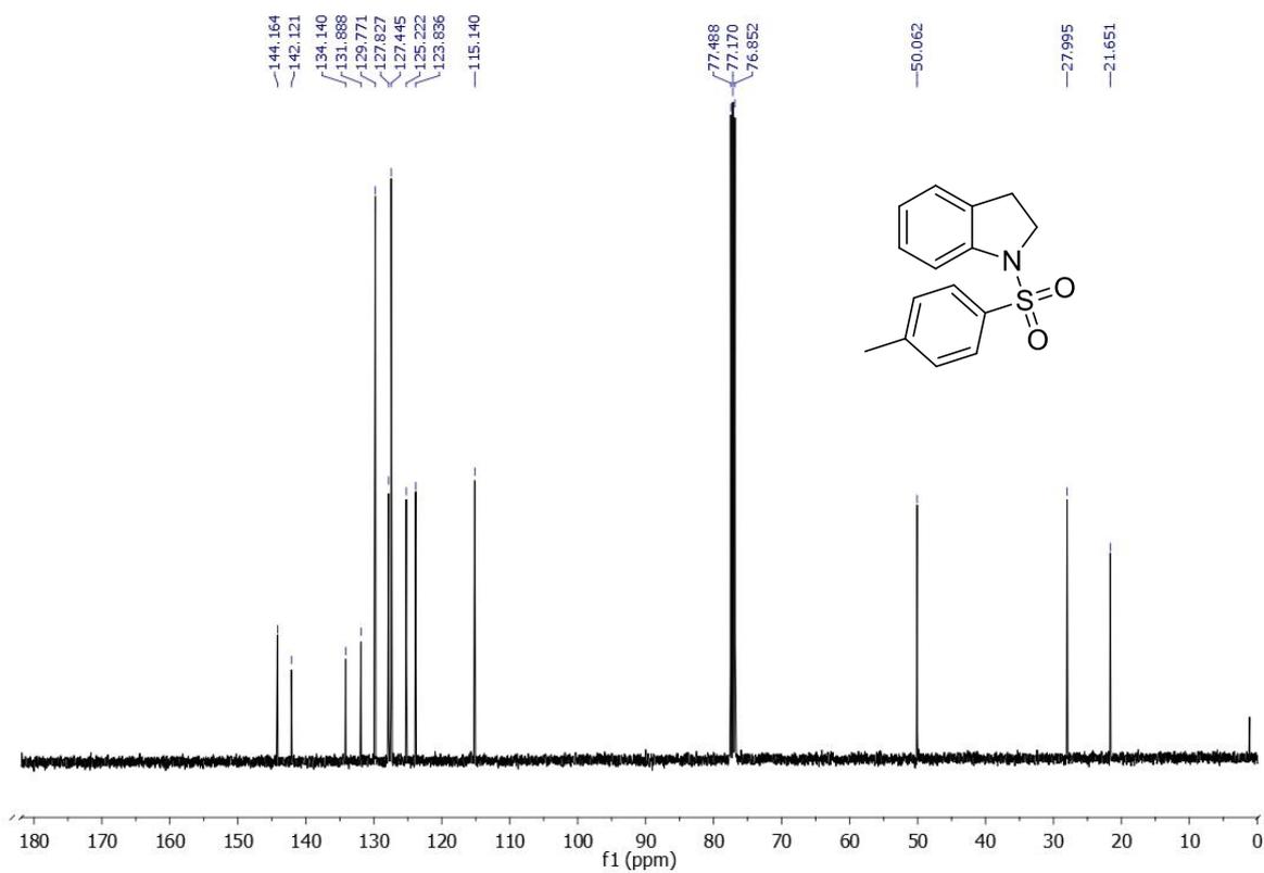
**Figure 3.88. <sup>13</sup>C NMR spectrum of 1-Tosylindoline (1i).**
