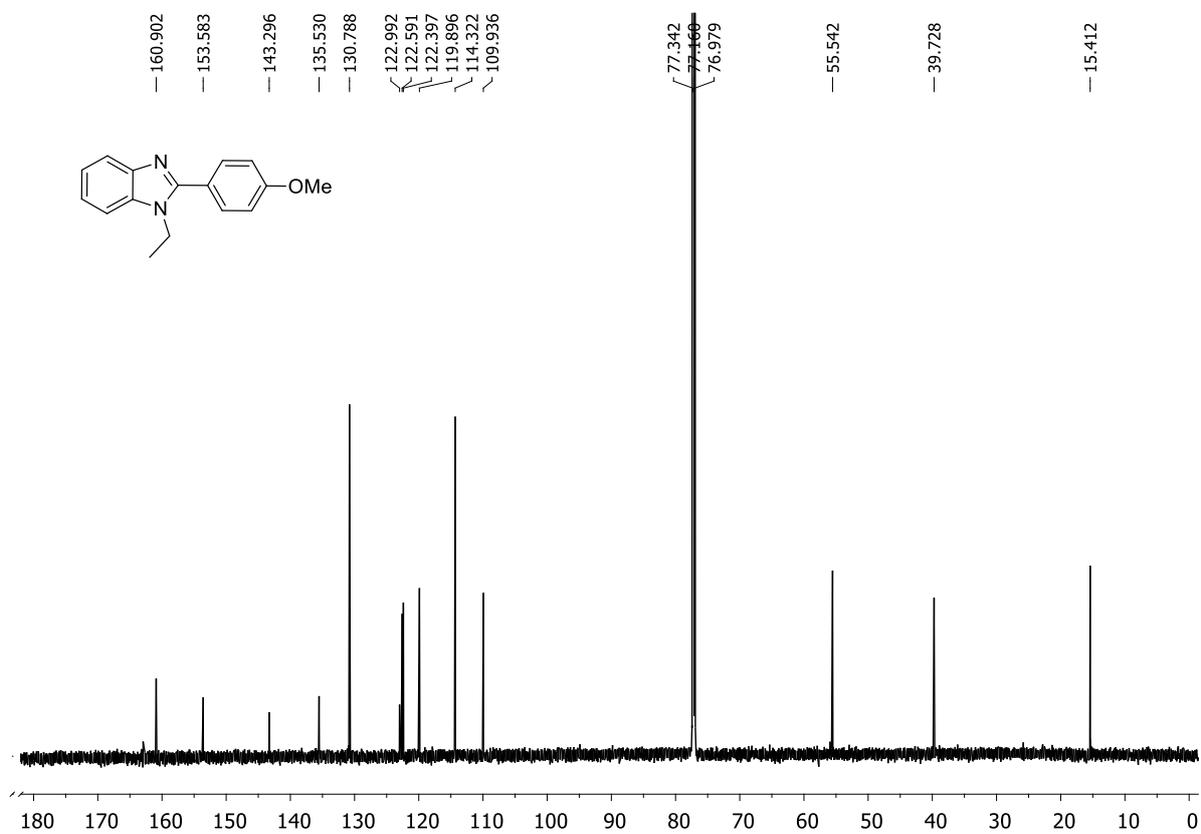
**Figure 5.21**  $^{13}\text{C}$  NMR of 1-Ethyl-2-(4-methoxyphenyl)-benzo[d]imidazole (**2h**)
