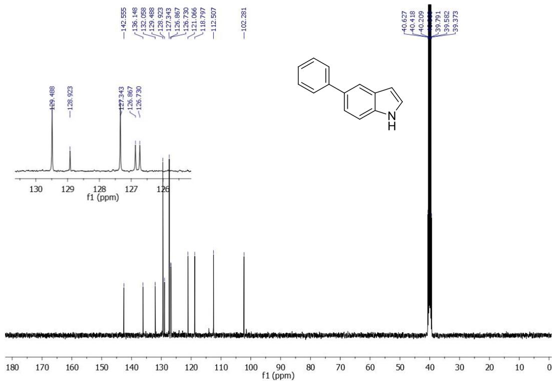
**Figure 3.60.** <sup>13</sup>C NMR spectrum of 5-Phenyl-1H-indole(1n').
