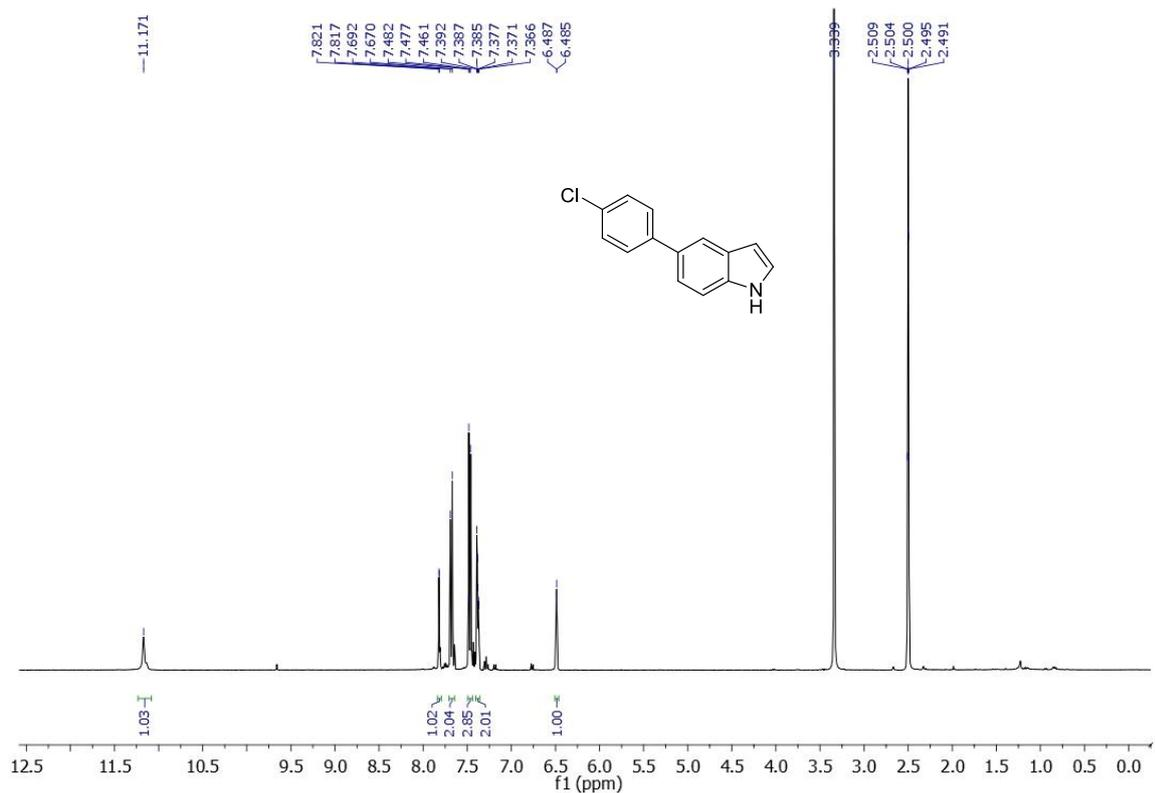
**Figure 3.69.** <sup>1</sup>H NMR spectrum of 5-(4-Chlorophenyl)-1H-indole (**1s'**).
