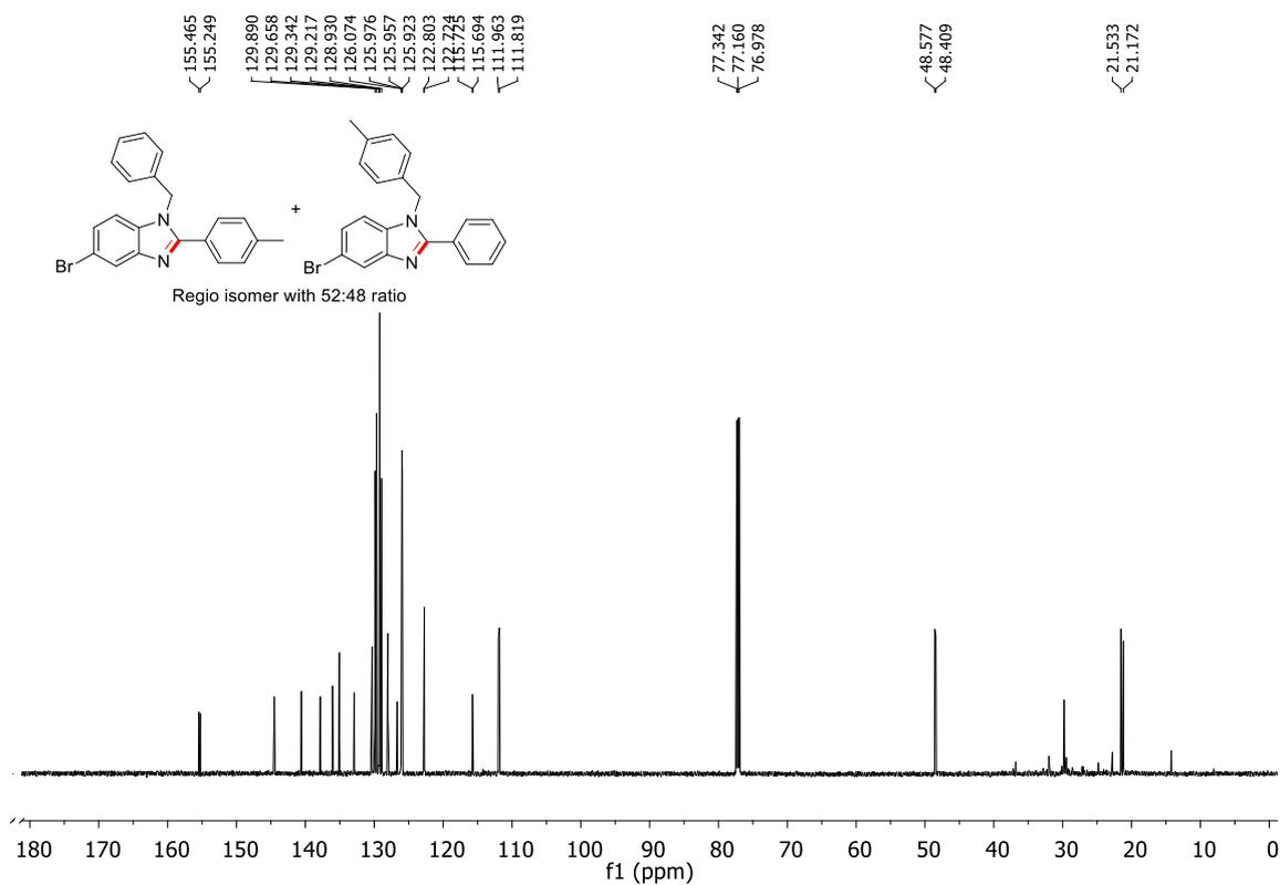
**Figure 4.83.**  $^{13}\text{C}$  NMR of 1-Benzyl-5-bromo-2-(p-tolyl)-benzo[d]imidazole and 5-Bromo-1-(4-methylbenzyl)-2-phenyl-benzo[d]imidazole (**2o**)
