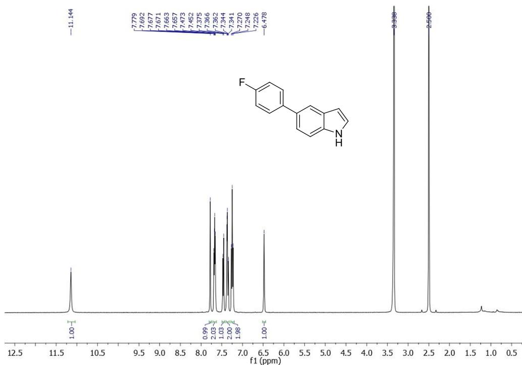
Figure 3.67.  $^1\text{H}$  NMR spectrum of 5-(4-Fluorophenyl)-1H-indole (**1r'**).
