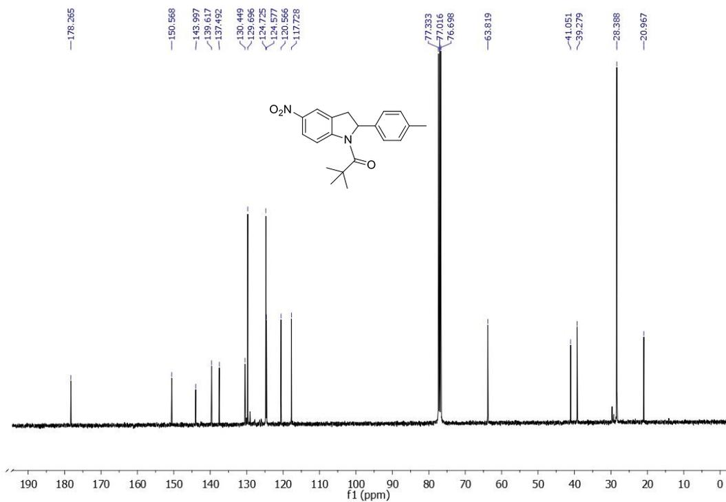
**Figure 3.18.** <sup>13</sup>C NMR spectrum of 2,2-Dimethyl-1-(5-nitro-2-(p-tolyl)indolin-1-yl)propan-1-one (**2f**).
