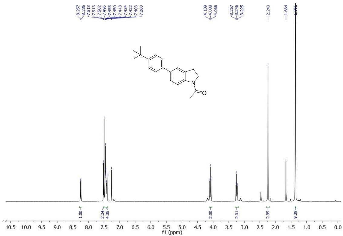
**Figure 3.97.** <sup>1</sup>H NMR spectrum of 1-(5-(4-(tert-Butyl)phenyl)indolin-1-yl)ethanone (**10**).
