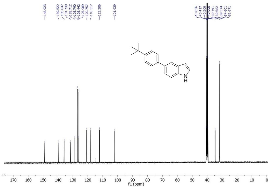
**Figure 3.62.** <sup>13</sup>C NMR spectrum of 5-(4-(tert-Butyl)phenyl)-1H-indole (**1o'**).
