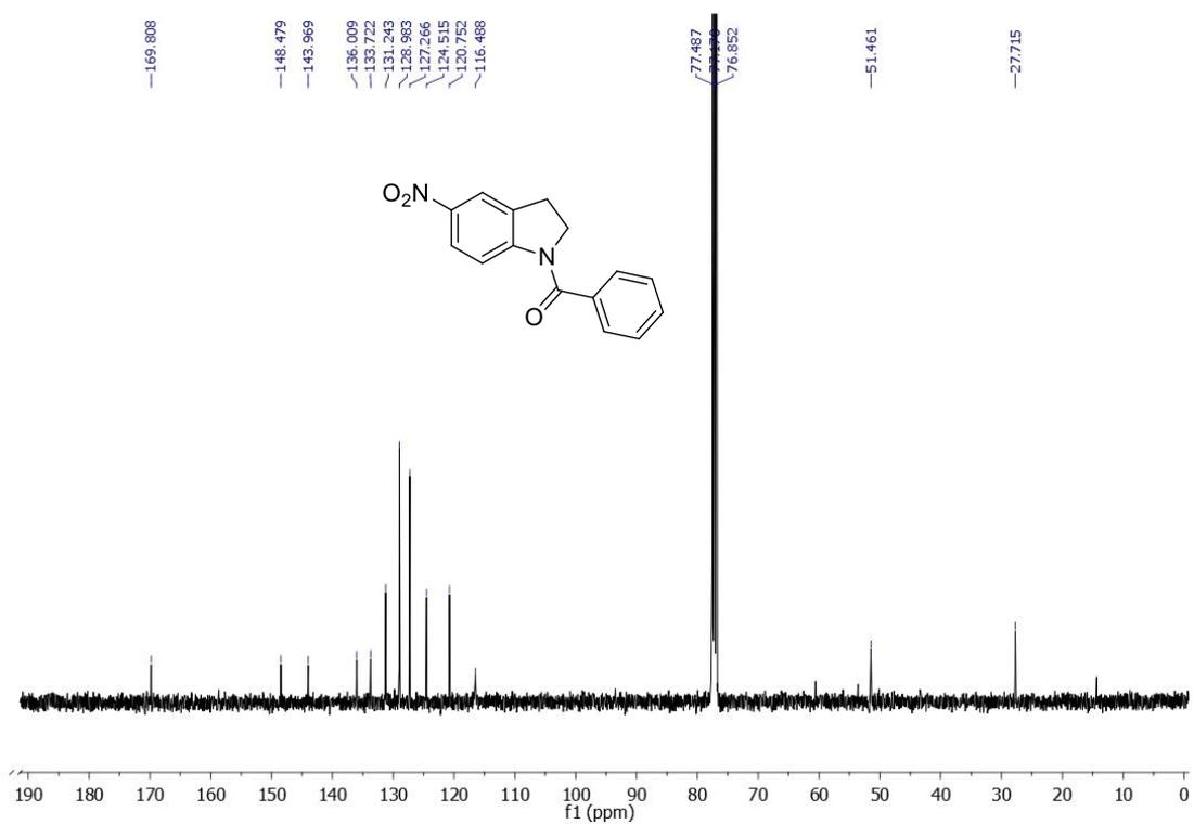
**Figure 3.26.** <sup>13</sup>C NMR spectrum of (5-Nitroindolin-1-yl)(phenyl)methanone (**2j**).
