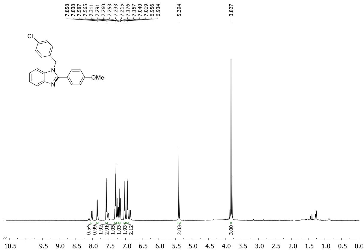
**Figure 5.36** <sup>1</sup>H NMR of 1-(4-chlorobenzyl)-2-(4-methoxyphenyl)-benzo[d]imidazole (2p)
