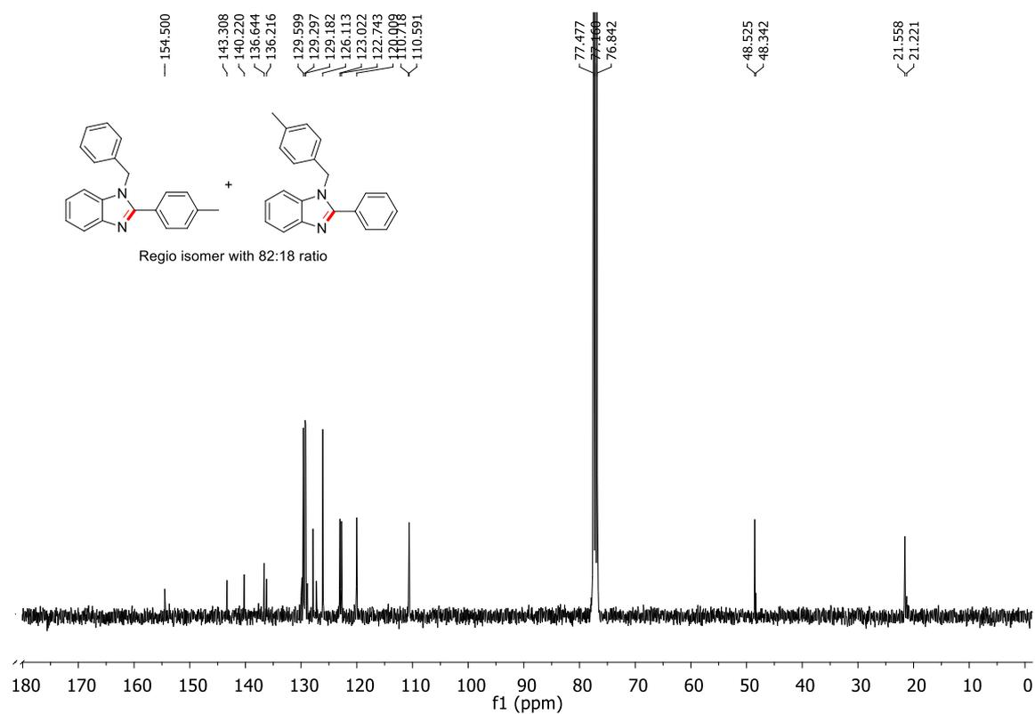
**Figure 4.81.** <sup>13</sup>C NMR of 1-Benzyl-2-(p-tolyl)-benzo[d]imidazole and 1-(4-Methylbenzyl)-2-phenyl-benzo[d]imidazole (**2n**)
