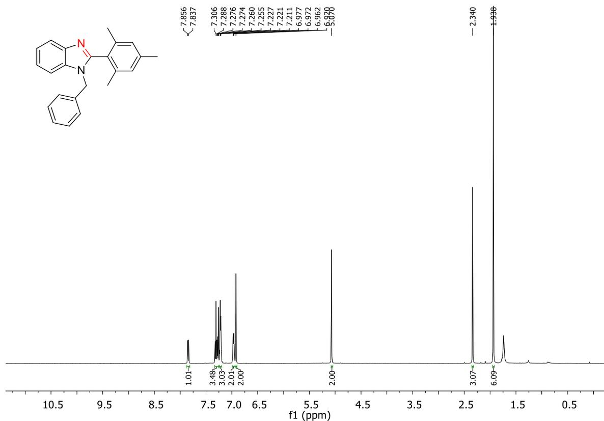
Figure 4.92.  $^1\text{H}$  NMR of 1-Benzyl-2-mesityl-benzo[d]imidazole (**2s**)
