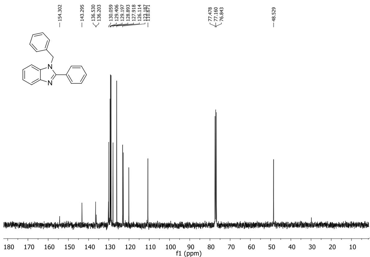
**Figure 4.55.** <sup>13</sup>C NMR of 1-Benzyl-2-phenyl-benzo[d]imidazole (**2a**)
