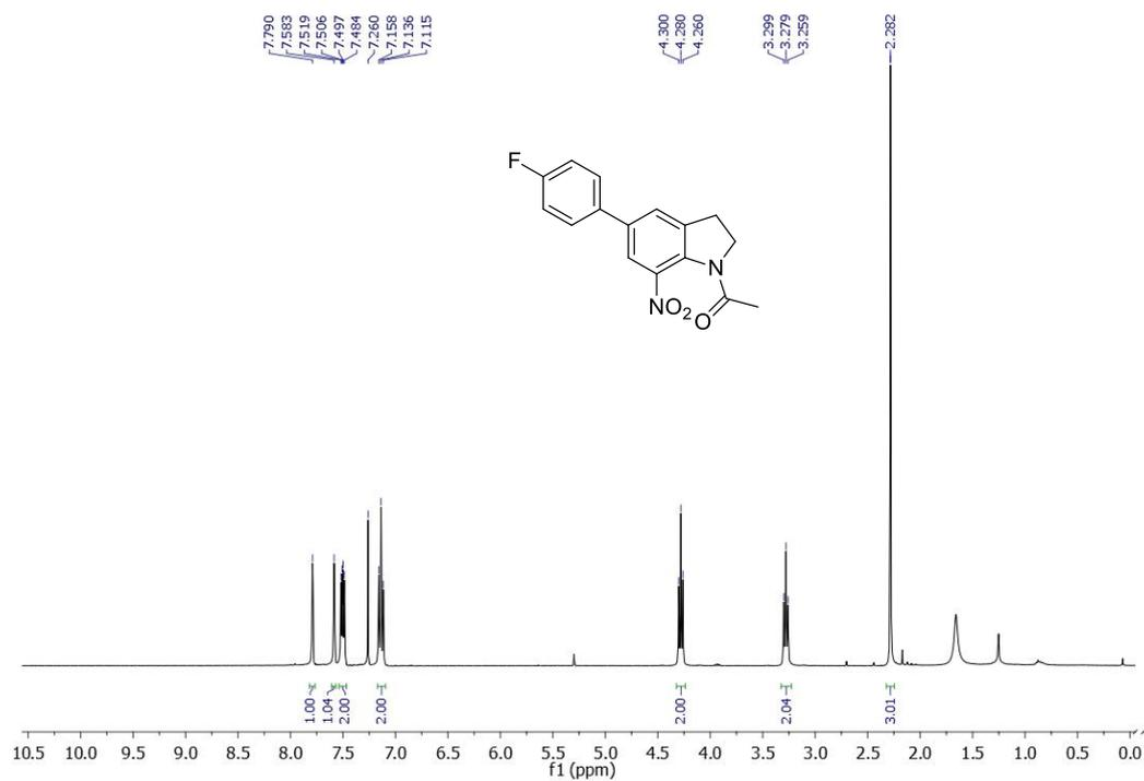
**Figure 3.41.** <sup>1</sup>H NMR spectrum of 1-(5-(4-Fluorophenyl)-7-nitroindolin-1-yl)ethanone (**2r**).
