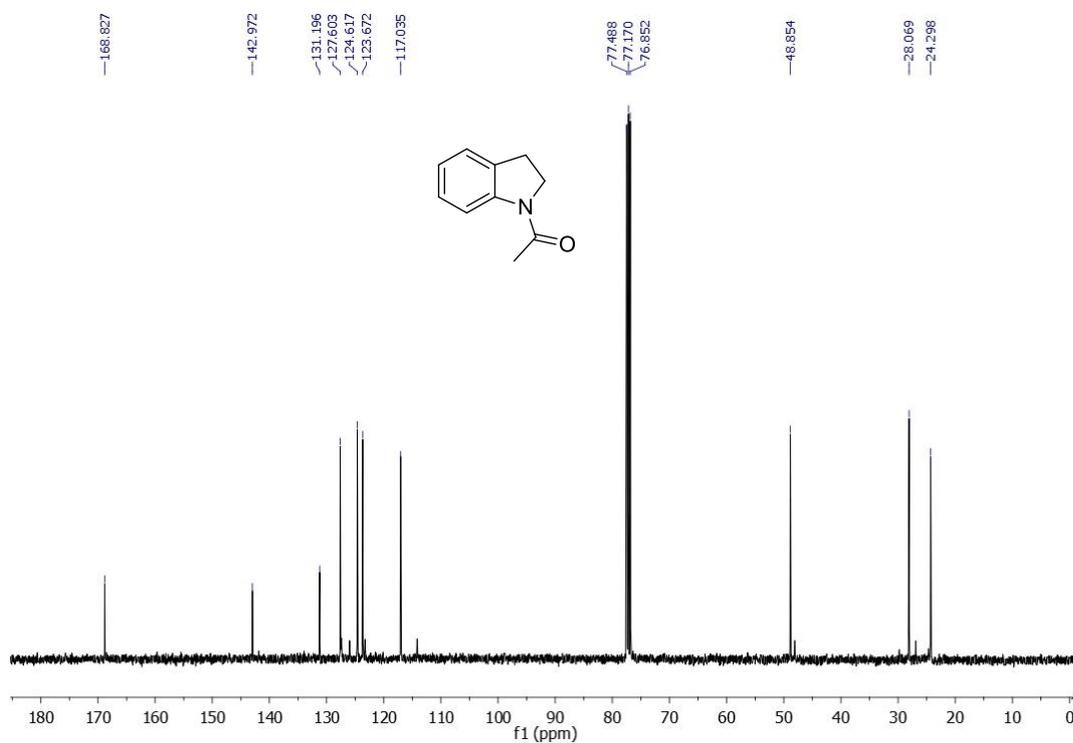
**Figure 3.72.**  $^{13}\text{C}$  NMR spectrum of 1-(Indolin-1-yl)ethanone (**1a**).
