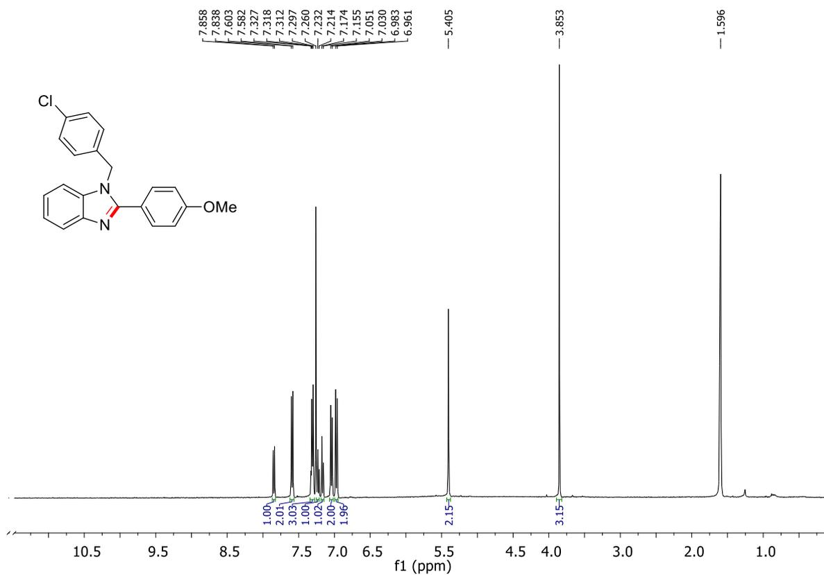
**Figure 4.100.** <sup>1</sup>H NMR of 1-(4-chlorobenzyl)-2-(4-methoxyphenyl)-benzo[d]imidazole (**2u**)
