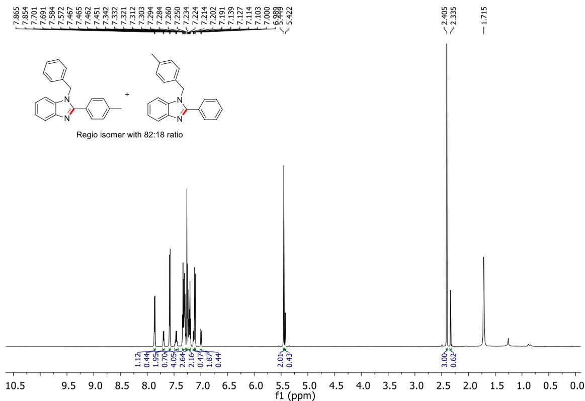
**Figure 4.80.** <sup>1</sup>H NMR of 1-Benzyl-2-(p-tolyl)-benzo[d]imidazole and 1-(4-Methylbenzyl)-2-phenyl-benzo[d]imidazole (**2n**)
