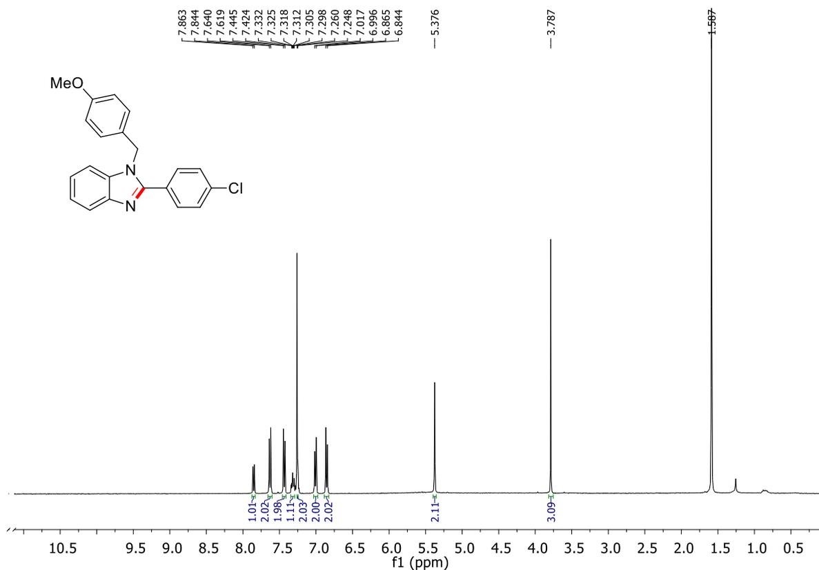
**Figure 4.102.** <sup>1</sup>H NMR of 2-(4-chlorophenyl)-1-(4-methoxybenzyl)-benzo[d]imidazole (**2u'**)
