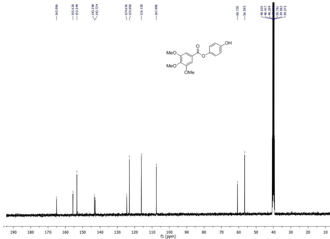
Figure 2.28.  $^{13}\text{C}\{^1\text{H}\}$  NMR spectrum of 4-hydroxyphenyl-3,4,5-trimethoxybenzoate (**31**).
