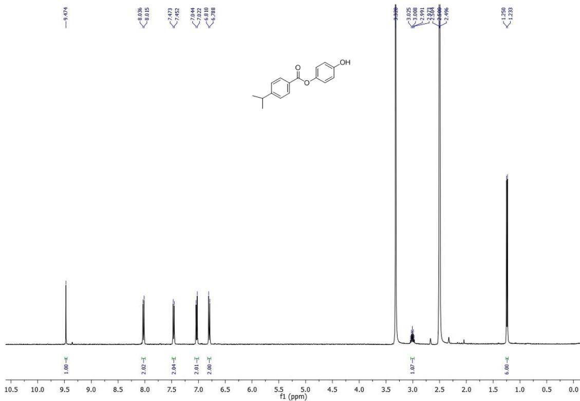
Figure 2.31. <sup>1</sup>H NMR spectrum of 4-hydroxyphenyl-4-isopropylbenzoate (3n).
