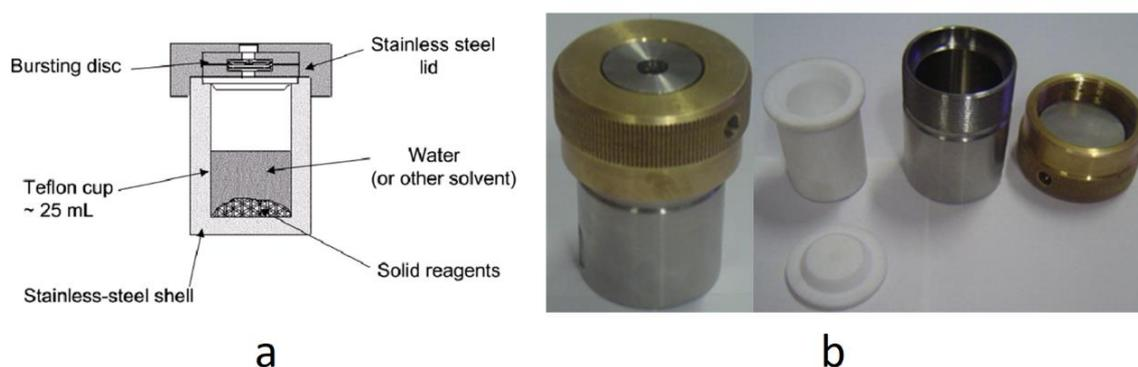
**Fig. 1.23.** (a) A schematic of Teflon<sup>TM</sup>-lined, stainless autoclave typically used in the laboratory and (b) The external view of the autoclave used for the synthesis described in this thesis with Teflon inserts<sup>106</sup>.
