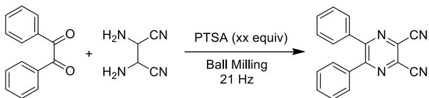
In a representative experimental procedure, benzil (0.5 mmol) and dicyanodiamine (0.5 mmol) were transferred to a 10 mL stainless steel jar equipped with grinding ball (15 mm
