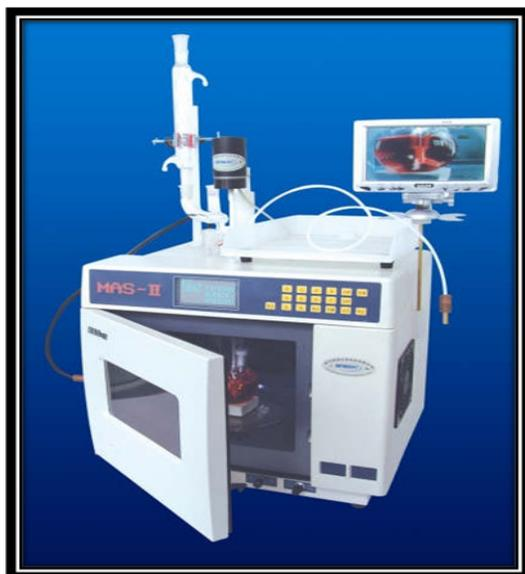
**Figure 2.1.** Photograph of microwave synthesizer.
