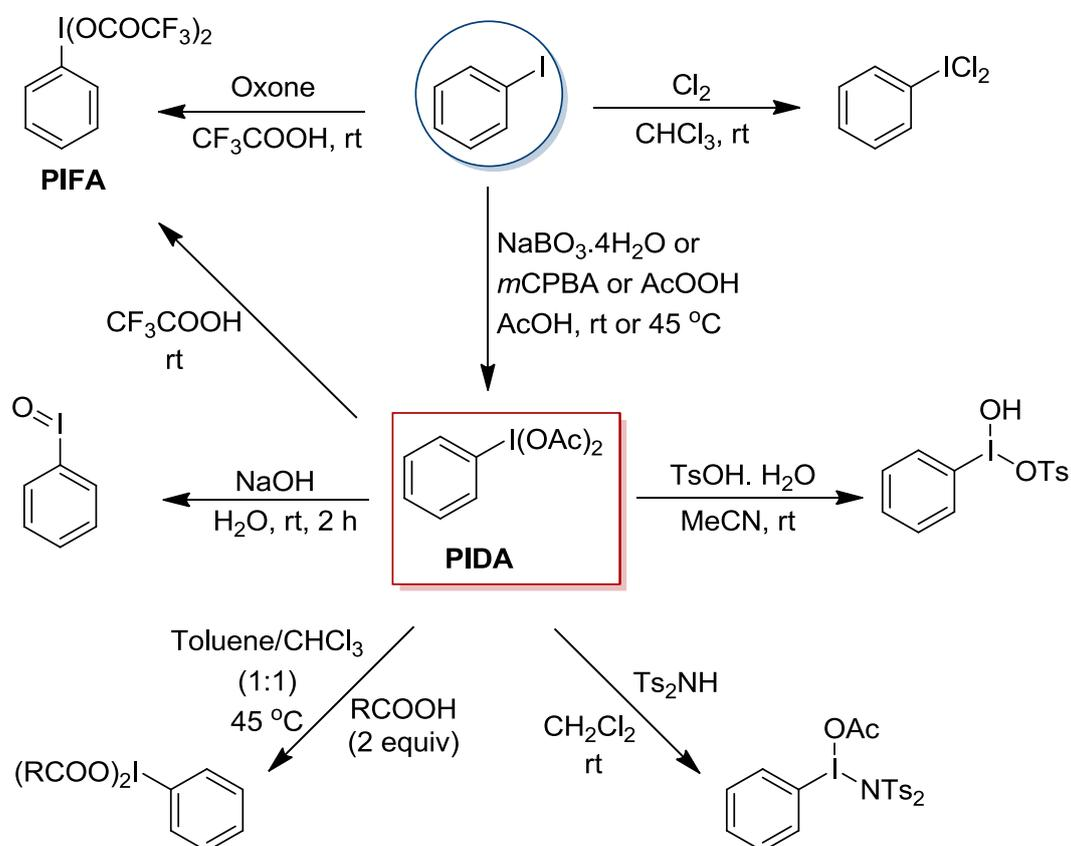
**Figure 1.2** Preparation of organoiodine(III) compounds.
