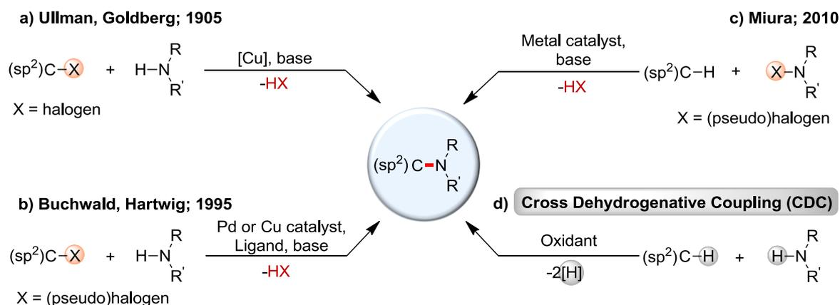
**Figure 1.8** Approaches for C(sp<sup>2</sup>)-N bond formation reactions.
