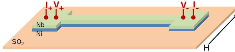
Figure 2.12: Schematic illustration showing an Ni/Nb bilayer stripe in four-probe geometry. An overlying Nb layer would directly sense the out-of-plane stray field of DWs of the Ni.
