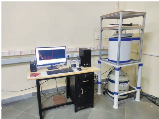
(HPGe detector that will be used in the NABL accredited radioanalytical laboratory)
