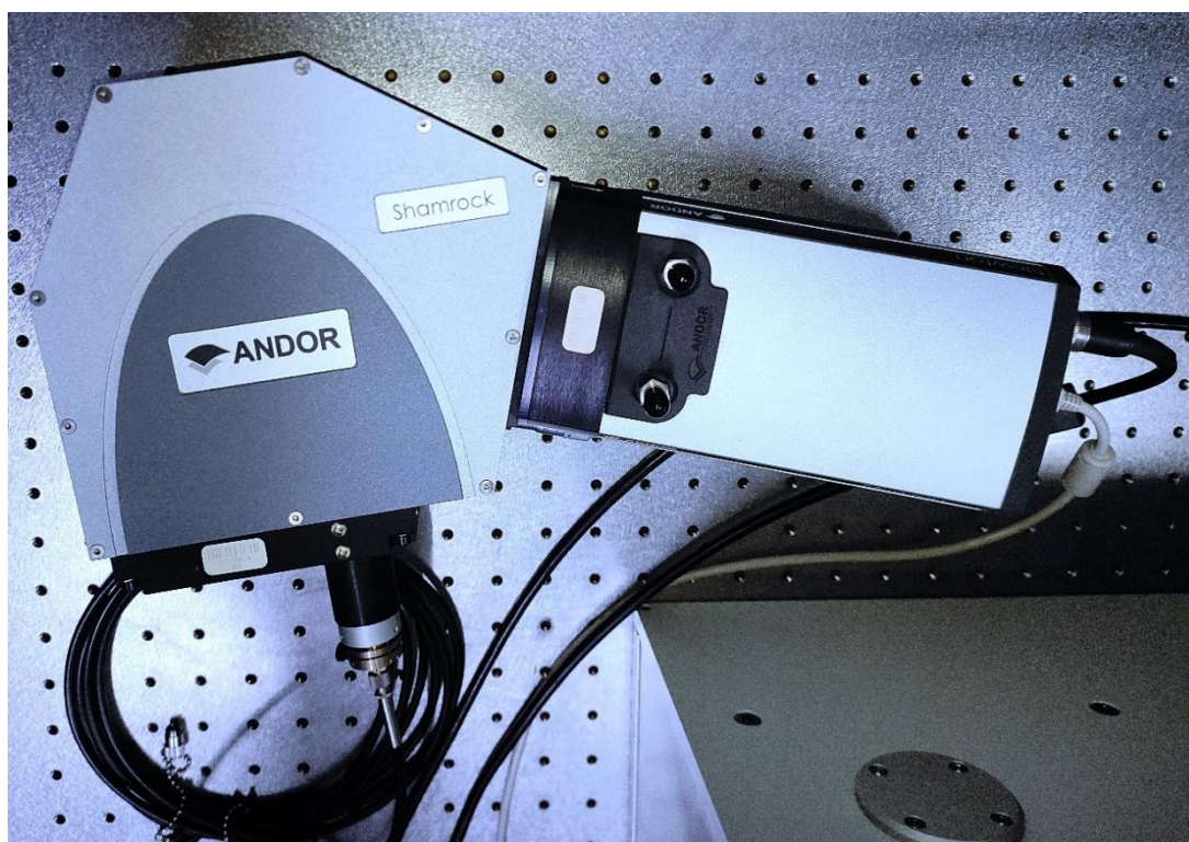
Figure 2.1 Spectrograph Instrument which is connected to our confocal fluorescence microscope.
