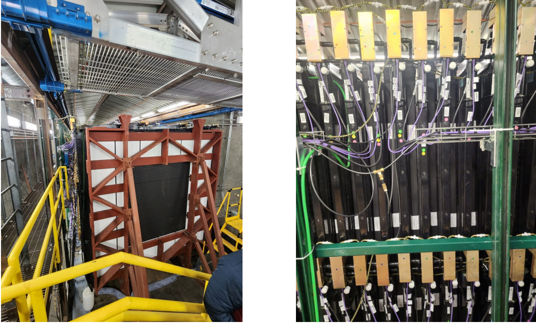
Figure 2.9: Recent photographs of the NOvA ND. The left panel shows the front view of the detector, while the right panel shows the detector electronics located at the top.
