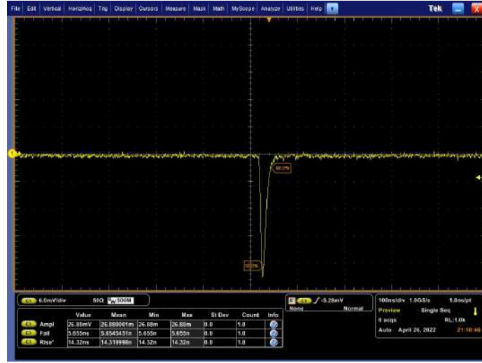
FIGURE 6.20: Example of a raw pulse recorded using an oscilloscope for an Am-Be source.
