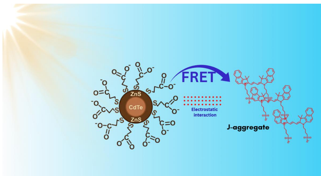
Scheme 5.1. Schematic representation of the interaction of CdTe@ZnS QDs with J-aggregate.
