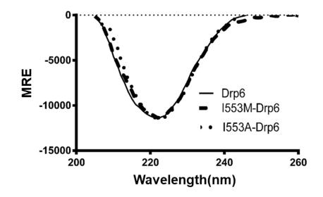
**Figure 3.3.5.1: Far UV-CD spectra of His-Drp6, His-Drp6-I553M and His-Drp6-I553A.** The graph shows the CD-spectra of His-drp6 (Drp6), His-drp6-I553M (Drp6-I553M) and His-drp6-I553A (Drp6-I553A). The spectra was recorded from 205nm to 260nm. Mean Residue Elipticity (MRE) was calculated using the formula mentioned in 3.2.1.7 and ploted against wavelength (nm).
