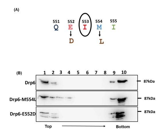
**Figure 3.3.7.1:** (**A**) **Scheme indicating the residues in the vicinity of I553.** The amino acid residues E552 was mutated to D and M554L was mutated to L.(**B**) **Liposome co-floatation** 97
