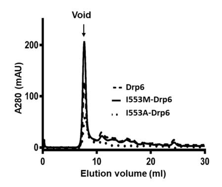
**Figure 3.2.4.2: Size exclusion chromatography of Drp6, I553M-Drp6 and I553A-Drp6.** Gel filteration of Drp6, I553M-Drp6 and I553A-Drp6 was performed using Superdex 200 10/300 GL column. All the three proteins eluted majorly in the void fraction. Arrow indicates the void volume.
