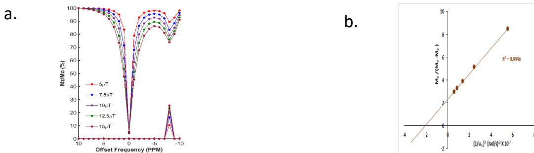
Figure 11 : (a) Dependence of CEST percentage on saturation field strength ranging from 5 \mu\text{T} to 15 \mu\text{T} for 8.3 pH (b) Omega plot for exchange rate measurement for pH 8.3. The expected linear relationship of M_z/(M_0 - M_z) as a function of 1/\omega_1^2 ( \text{rad/sec})^{-2} \times 10^{-7} was obtained at 9.4 T of 12.5 mM compound in 0.1M Tris-HCl buffer. RF presaturation pulse was applied for 6 s ensuring complete saturation.
