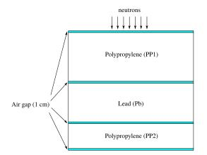
Figure 5.19: Rectangular shielding layers used for simulation [5]. The thicknesses of Pb and PP2 are varied.
