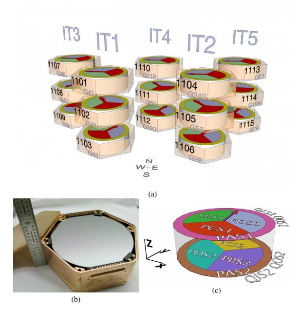
Figure 2.3: (a) SuperCDMS detectors stacked in five towers, with each containing three germanium detectors [5]. (b) a single detector module inside a copper housing [5]. (c) a cartoon that shows the phonon and charge channels on each side of the detector [5].
