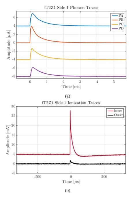
Figure 2.4: (a) Phonon output traces from the four channels on side 1 (top surface) of iT2Z1 for an example event [3]. For clarity, the amplitudes of the traces from the channels are vertically shifted by 4 nA. The traces from inner and outer ionization chanels of side 1 of iT2Z1 for an example event [3]. For clarity, the inner channel's trace is shifted upwards by 5 mV. See phonon and charge chanels in Fig. 2.3 (c).
