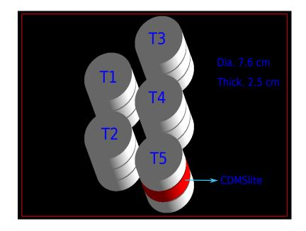
Figure 4.19: The simulation geometry defined with GEANT4 for the singles-cut efficiency calculation. The detectors are stacked in five towers with each having three detectors. The detector in red is the CDMSlite detector. LIPs are thrown isotropically or with an angular distribution of  $\cos^2 \theta$  shape towards this detectors' arrangement.
