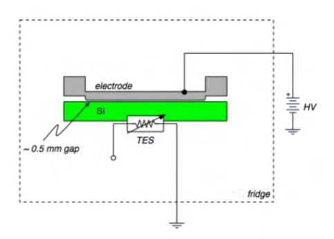
FIGURE 2.7: A schematic of the detector showing one face covered with TES to measure phonons produced in the crystal. The phonon sensors are held at the ground potential and the crystal is biased through a vacuum gap using an aluminum electrode.
