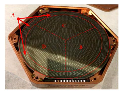
FIGURE 2.6: A picture of the 100 g silicon detector (diameter=7.5 cm and thickness=1 cm) used in this work kept inside a copper casing. The phonon sensors consist of ~1000 TES sensors. The TES sensors are divided into 4 groups of ~250 sensors and independently read out forming 4 channels (A, B, C, and D). This configuration allows reconstruction of interaction locations based on the relative amplitudes and time delays between independent channels.
