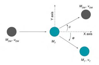
FIGURE A.1: A schematic showing the kinematic of the elastic scattering process between a dark matter particle and a target nucleus.
