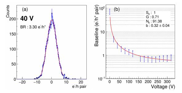
FIGURE 2.14: (a) The noise energy distribution in  $e^-/h^+$  pair energy scale is shown. The sigma of the Gaussian fit is the baseline resolution of the detector. Supplementary figures showing the noise energy distribution at all remaining bias voltages can be found in Appendix C. (b) Baseline resolution in units of  $e^-/h^+$  pair units as a function of voltage. The data points are fit to a functional form given by N/S where N and S are defined in Eq. 2.10 and Eq. 2.11 respectively [16].
