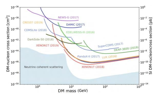
FIGURE 1.8: The results of several dark matter search experiments shown in the DM-nucleon vs DM mass parameter space. The region above a solid curve corressponding to an experiment has been excluded by it. The region below the solid curves is yet to be explored. The shaded region at the bottom of the figure corresponds to a phenomena called as coherent elastic neutrino nucleus scattering [29]. Figure taken from PDG 2020 [30].
