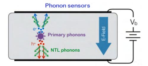
FIGURE 2.3: A schematic of the detector. The scattering process and associated primary phonons are shown in violet. The electrons are shown in blue dots and holes in red dots. The NTL phonons from the charge carriers as they drift along the electric field are shown in green.
