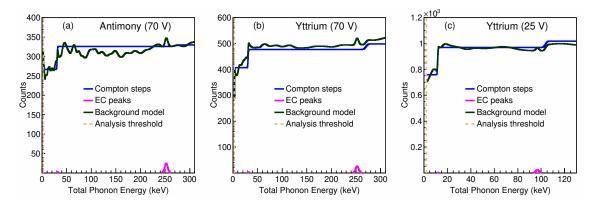
FIGURE 3.12: The different components of the background model are shown. Panel (a) is for the <sup>124</sup>Sb data at 70 V, panel (b) is for <sup>88</sup>Y data at 70 V, and panel (c) is for <sup>88</sup>Y data at 25 V. The final background model after incorporating the residuals in the fit from the Comptons and EC peaks to neutron-OFF data is shown in dark green [27].
