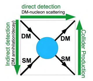
FIGURE 1.6: A schematic diagram to symbolize the three types of DM search mechanisms. The green arrows indicate the direction from participants to products in an interaction. The blue region symbolizes a mediator for the process. Here DM stands for dark matter particle and SM stands for standard model particle [20].
