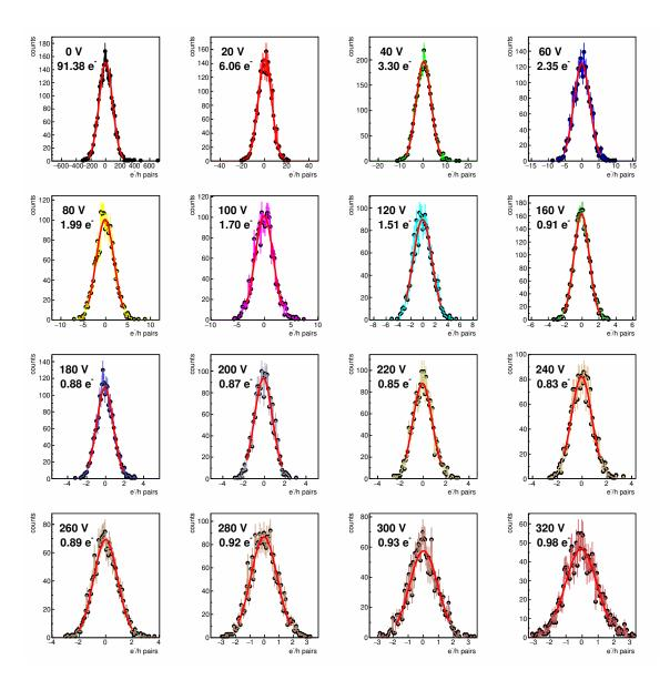
FIGURE C.2: The baseline resolution obtained by fitting a Gaussian (solid red line) to the noise energy distribution (black markers) in units of  $e^{-}/h^{+}$  pairs from 0 V to 320 V.
