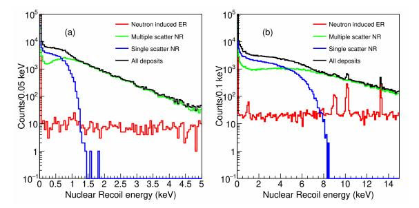
FIGURE 3.9: The simulated recoil energy distributions in (a) <sup>124</sup>Sb+<sup>9</sup>Be, and (b) <sup>88</sup>Y+<sup>9</sup>Be in the detector T5Z2. The energy depositions from electron recoils (ER) that come from gammas is shown in red, the energy depositions from multiple scattered neutrons in the detector is shown in green. The energy distribution of single scatter neutrons is shown in blue [27].
