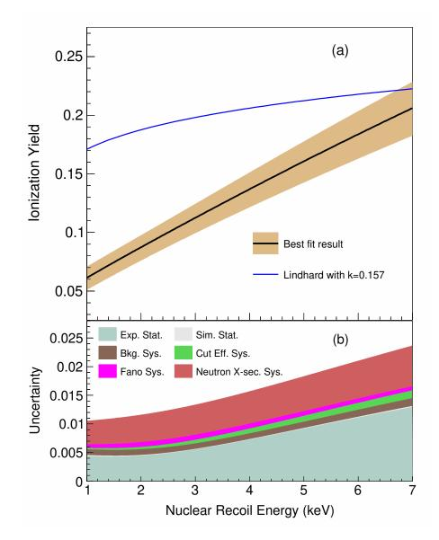
FIGURE 3.14: (a) The ionization yield from the best fit values of the 2 k-parameter Lindhard model as a function of the nuclear recoil energy in germanium. Blue line shows the classic Lindhard model with k = 0.157 (b) The contribution of various sources of statistical and systematic uncertainties to the ionizzation yield in germanium [27].
