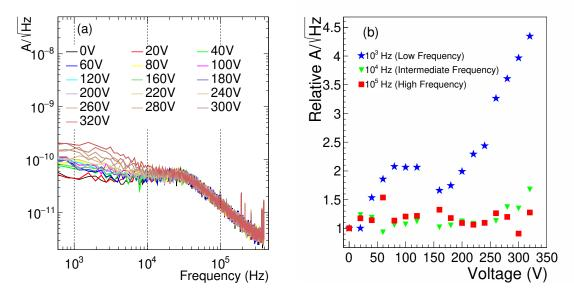
FIGURE 2.12: (a) The (TES current amplitude)/ $\sqrt{\text{Hz}}$  plotted as a function of frequency for different voltages from 0 V to 320 V. These distributions are the phonon noise PSDs. (b) The ratio of the noise PSD at 0 V to the noise PSDs at every other voltage is shown at three chosen frequencies; low, intermediate and high, to assess the phonon noise performance of the detector.
