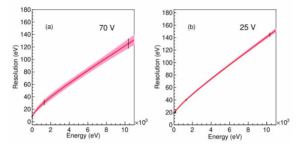
FIGURE 3.11: (a) The resolution of the T5Z2 detector operated at 70 V as a function of energy. The resolutions of the K, and L shell gammas were used as the data points for fitting of the resolution model. The M shell peak was not visible in the 70 V datasets, (b) The resolution of the T2Z1 detector operated at 25 V as a function of energy. The K, L and M shell resolutions were taken as the data points for fitting of the resolution model [27].
