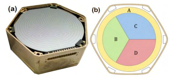
FIGURE 3.4: (a) A Germanium SuperCDMS detector in its Copper housing [28], (b) A schematic of the detector with the phonon channel layout [29].
