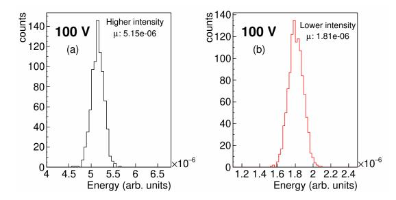
FIGURE 2.11: The laser energy distribution and their means  $(\mu)$  in arb. units is shown for the higher intensity laser at 100 V bias in panel (a) and the lower intensity laser at 100 V bias in panel (b).
