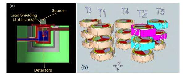
FIGURE 3.3: (a) A GEANT4 schematic of the experimental setup with the shielding configuration.
