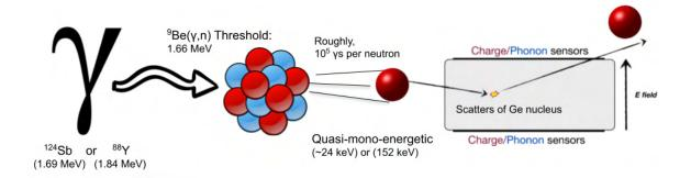
FIGURE 3.2: A schematic representation of the method used to obtain the ionization yield in Ge by the SuperCDMS experiment.
