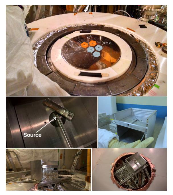
FIGURE 3.5: (a) Top view of the SuperCDMS Soudan ice box, (b) top view of the gamma source rod with the <sup>9</sup>Be wafer underneath. The gamma source is placed within the source rod, (c) the source box with the detachable source rod, (d) side view of the source box with the lead shielding to counter the high gamma rate from the source, and (e) top view of the source box placed on a bridge above detector towers 2 and 5.
