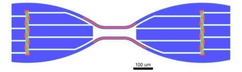
FIGURE 2.5: A schematic of the two TESs connected in a chain is shown. The blue region is Al. The red regions are W. The contact between the two Al fins of the TES on either side are shown in pink. Figure from Ref. [14]
