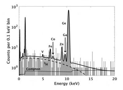
FIGURE 4.7: The best fit result for each background source to the CDMSlite energy distribution using the negative log likelihood method. The dashed line shows the <sup>3</sup>H PDF fit result using NLL. The dotted line shows the best fit for the compton steps. The solid line shows the best fit PDF for all the EC peaks in Ge [19].
