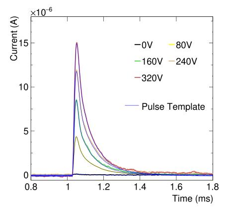
FIGURE 2.10: The phonon raw pulses as current signals in the TES as a function of bias voltages is shown. The pulses below 100 V were at a laser intensity of ~ 1150 eV. The pulses above 100 V in the figure have been scaled to data below 100 V by a factor of 2.85. The pulse template fit to the pulses using the optimal filter (OF) method is also shown [16]
