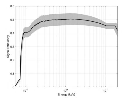
FIGURE 4.5: The signal efficiency as a function of energy. The  $1\sigma$  uncertainty on the efficiency is shown by the shaded region [19].
