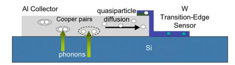
FIGURE 2.4: A schematic of the capture process of the phonons in the TES technology is shown. The while circles are the quasiparticles produced in Al and blue circles are quasiparticles produced in W [10].
