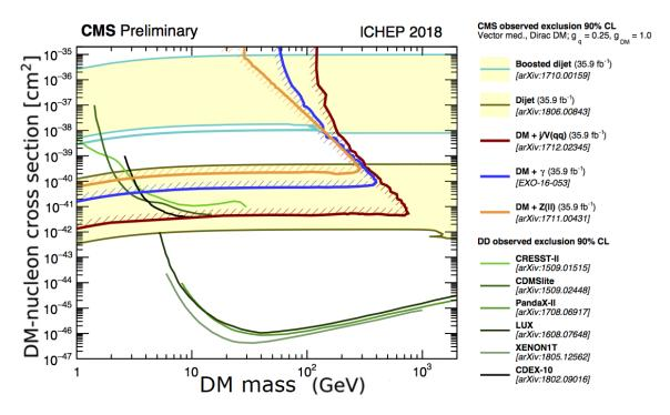
FIGURE 1.9: The search results from direct DM search experiments are compared with results by the CMS experiment at CERN in the DM nucleon vs DM mass parameter space [31]
