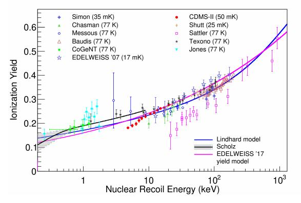
FIGURE 3.1: World data on ionization yield measurements as a function of recoil energies in Ge [3–15]. Measurements by Schutt, Simon, EDELWEISS, CDMS-II and Scholz are in the mK scale temperature, while all others are at 77 K. The prediction by Lindhard et. al. [16–20] has also been shown for comparison.
