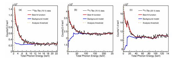
FIGURE 3.13: Energy spectrum for the three data sets, (a) <sup>124</sup>Sb+<sup>9</sup>Be with T5Z2 biased at 70 V, (b) <sup>88</sup>Y+<sup>9</sup>Be with T5Z2 biased 70 V and (c) <sup>88</sup>Y+<sup>9</sup>Be with T2Z1 biased at 25 V, with best fit result overlaid, shaded area shows the fit uncertainty. Blue curve shows the fitted gamma background contribution [27].
