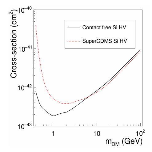
FIGURE 5.1: A comparison of the sensitivity curves between the SuperCDMS SNOLAB Si HV detectors (red dashed line), and the contact free Si HV detectors (solid black line) discussed in this thesis. The curves were made assuming the <sup>3</sup>H contamination levels discussed in this thesis.
