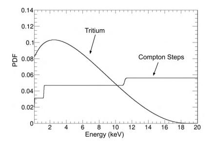
FIGURE 4.6: A PDF of the <sup>3</sup>H beta decay and the Compton step model.
