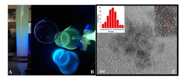
**Figure 3.1.** (A) Visual silica column separation of as-synthesized FCD under UV illumination (~365 nm). (B) Two subsets, BFCD and GFCD obtained after visual silica column separation. A third beaker containing only water was placed close to the UV lamp for comparison with the other two FCD solutions. (C) HR-TEM image of a BFCD particle and the particle size distribution. GFCD shows a similar TEM image and particle size distribution.
