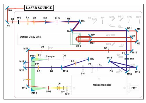
**Scheme 2.4.** Schematic representation of the upconversion setup, Fluomax from IB photonics. In the scheme, the red line corresponds to the fundamental laser beam and the blue one frequency-doubled visible beam.
