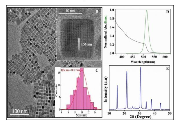
**Figure 7.1.** (A) TEM images of CsPbBr<sub>3</sub> NCs. (B) HR-TEM image of a CsPbBr<sub>3</sub> NC. (C) Particle size distribution of the NCs, the center of mass of which is located at 10 nm. (D) Absorption (black) and emission (green,  $\lambda_{ex}$ =400 nm) spectra of CsPbBr<sub>3</sub> NCs in toluene. (E) XRD spectrum of CsPbBr<sub>3</sub> NCs, which shows the cubic phase of the crystals.
