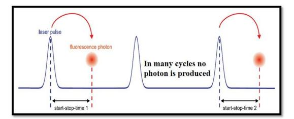
Scheme 2.1. The working principle of TCSPC setup.<sup>[119]</sup>
