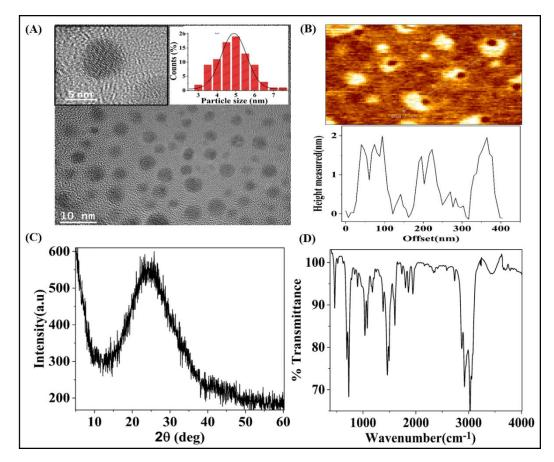
**Figure 6.1.** (A) Particle size distribution of GQDs obtained from the HRTEM study. (B) Topological height of the GQDs is measured to be ~1.8 nm from the AFM study, indicating the presence of ~4-5 graphene layers. (C) Powder XRD spectrum of GQDs. (D) FTIR spectrum of GQDs shows the presence of different organic functional groups on the surface.
