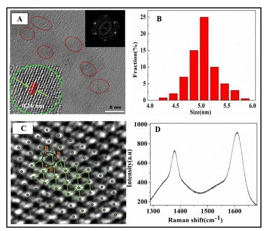
**Figure 4.1.** (A) HR-TEM image of GQDs. Insets show the FFT patterns and lattice spacings. (B) Size distribution of GQD particles, measured through HR-TEM. (C) Zoomed image (HR-TEM) of GQD surface to the atomic level. (D) Raman spectrum of GQDs.
