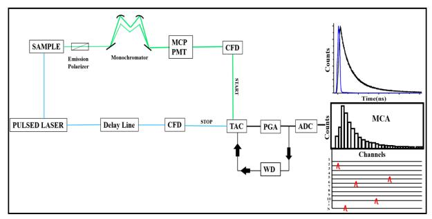
Scheme 2.2. Scheme representing a basic reverse mode TCSPC setup.
