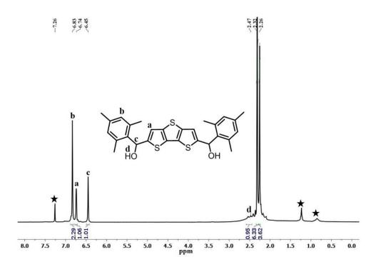
Figure 2.3.2: <sup>1</sup>H NMR spectrum of 6 in CDCl<sub>3</sub>. "Asterisk symbols are for impurities"
