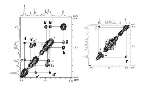
Figure 6.9: <sup>1</sup>H-<sup>1</sup>H COSY spectrum of 17a heterocyclic ring protons in CDCl<sub>3</sub>.
