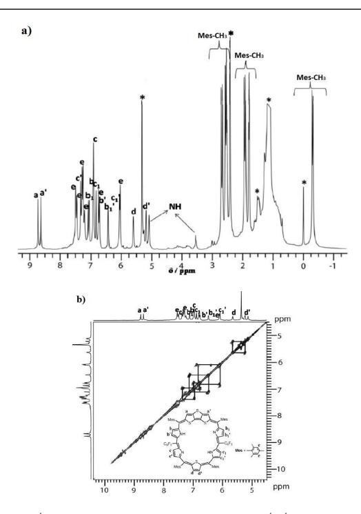
Figure 4.7: <sup>1</sup>H NMR spectrum of 28 at 183K in CD<sub>2</sub>Cl<sub>2</sub> (a) and <sup>1</sup>H-<sup>1</sup>H COSY spectrum of 28 with thiophene and pyrrolic  $\beta$ -CH proton correlations (b).
