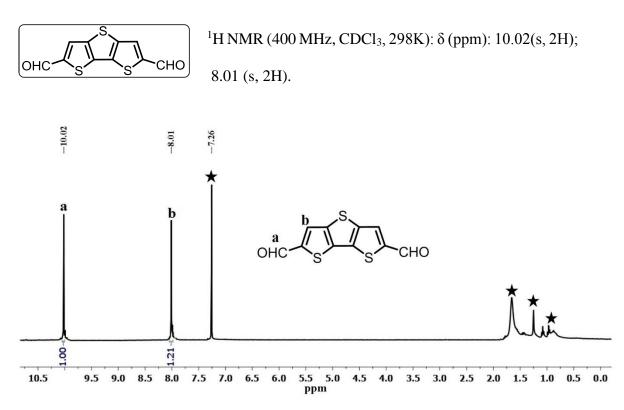
Figure 2.3.1: <sup>1</sup>H NMR spectrum of 5 in CDCl<sub>3.</sub> "Asterisk symbols are for impurities"
