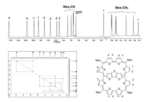
Figure 5.20: <sup>1</sup>H NMR and <sup>1</sup>H-<sup>1</sup>H COSY spectrum of 30a with heterocyclic ring
