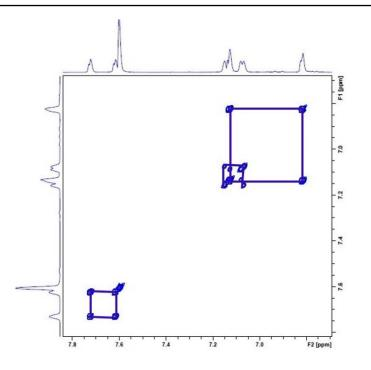
**Figure 3.13**: <sup>1</sup>H-<sup>1</sup>H COSY spectrum of **42** with correlation in pyrrole and thiophene rings.
