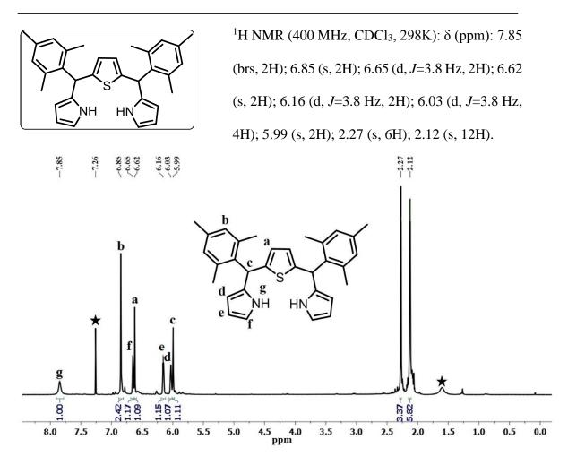
Figure 2.3.10: <sup>1</sup>H NMR spectrum of 17 in CDCl<sub>3.</sub> "Asterisk symbols are for impurities"
