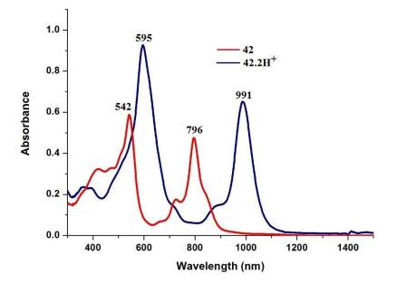
Figure 3.15: The electronic absorption spectrum of 42 and 42.2H<sup>+</sup> in CH<sub>2</sub>Cl<sub>2</sub>.
