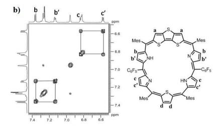
**Figure 4.4**: <sup>1</sup>H NMR spectrum of **28** at 298K in CDCl<sub>3</sub> (a) and <sup>1</sup>H-<sup>1</sup>H COSY spectrum of **28** with pyrrolic  $\beta$ -CH proton correlations (b).
