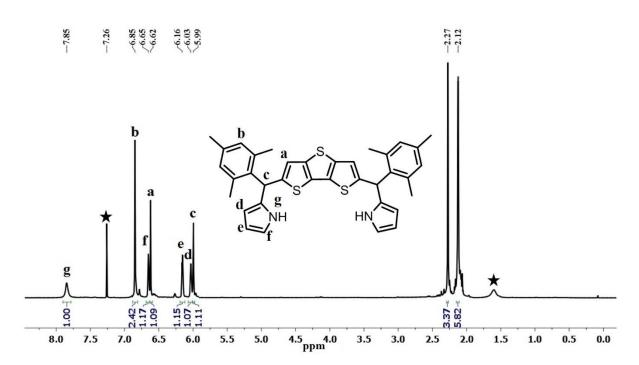
Figure 2.3.4: <sup>1</sup>H NMR spectrum of 8 in CDCl<sub>3</sub>. "Asterisk symbols are for impurities"
