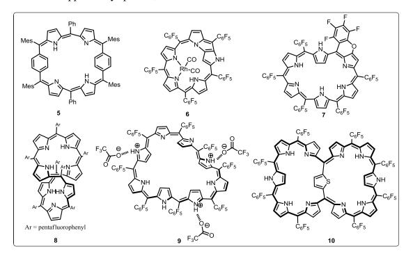
Figure 1.2: Examples of Möbius aromatic expanded porphyrins
