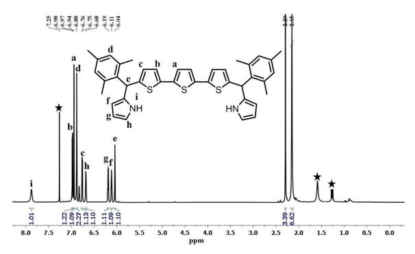
Figure 2.3.9: <sup>1</sup>H NMR spectrum of 14 in CDCl<sub>3.</sub> "Asterisk symbols are for impurities"
