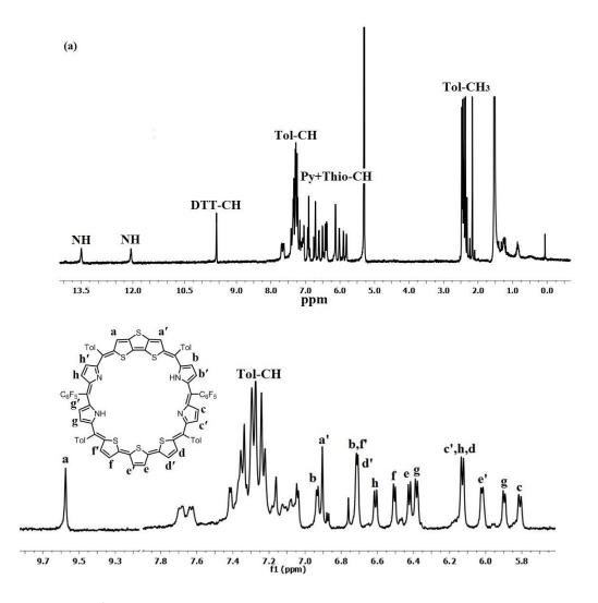
Figure 6.12: <sup>1</sup>H NMR spectrum of 17b in CD<sub>2</sub>Cl<sub>2</sub> (a). The expansion in aromatic ring
