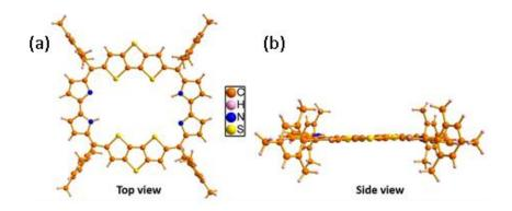
Figure 4: Structure of fused DTT octaphyrin 10: (a) Top view, (b) Side view.
