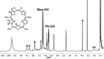
Figure 3.6: <sup>1</sup>H NMR spectrum of 38 with 4.5 equiv. of TFA in CD<sub>2</sub>Cl<sub>2</sub>.
