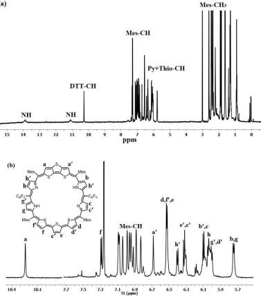
Figure 6.8: <sup>1</sup>H NMR spectrum of 17a in CDCl<sub>3</sub> (a). The expansion in aromatic ring
