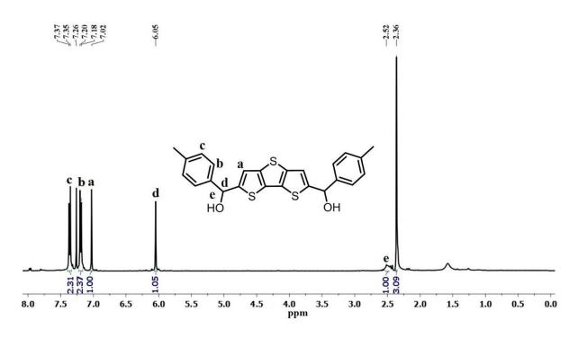
Figure 2.3.3: <sup>1</sup>H NMR spectrum of 7 in CDCl<sub>3</sub>
