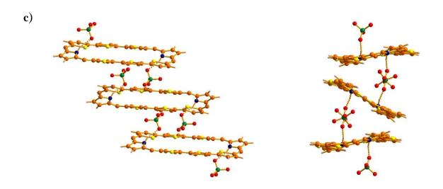
**Figure 5.12**: Single crystal X-ray structure of **26a.2H**<sup>+</sup> with intermolecular hydrogen bonding interaction with perchlorate anion. (a) Top view; (b) side view and (c) one-dimensional array.
