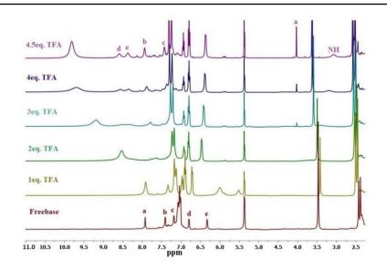
Figure 3.7: <sup>1</sup>H NMR titration experiment of 38 with dilute solution of TFA in CD<sub>2</sub>Cl<sub>2</sub>
