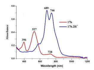
Figure 6.6: The electronic absorption spectrum of 17b and 17b.2H<sup>+</sup> in CH<sub>2</sub>Cl<sub>2</sub>.
