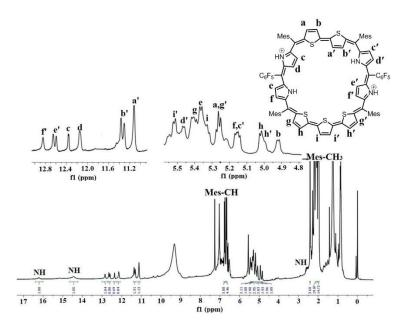
Figure 6.17: <sup>1</sup>H NMR spectrum of 18.2H<sup>+</sup> in CD<sub>2</sub>Cl<sub>2</sub>. The inset shows the expansion
