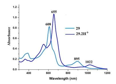
Figure 4.18: The electronic absorption spectrum of 29 and 29.2H<sup>+</sup> in CH<sub>2</sub>Cl<sub>2</sub>.
