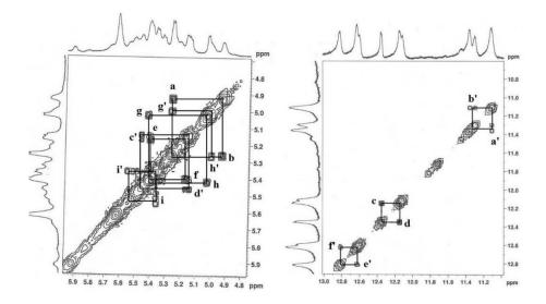
Figure 6.18: <sup>1</sup>H-<sup>1</sup>H COSY spectrum of 18.2H<sup>+</sup> aromatic ring protons in CD<sub>2</sub>Cl<sub>2</sub>.
