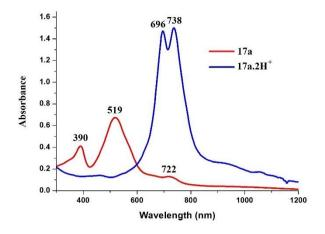
Figure 6.5: The electronic absorption spectrum of 17a and 17a.2H<sup>+</sup> in CH<sub>2</sub>Cl<sub>2</sub>.
