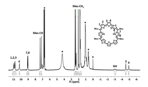
Figure 5.9: <sup>1</sup>H NMR spectrum of 26a.2H<sup>+</sup> in Toluene-d<sub>8</sub>
