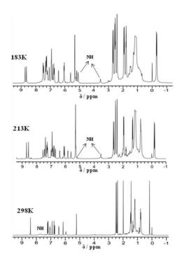
Figure 4.6: Variable temperature <sup>1</sup>H NMR spectrum of 28 in CD<sub>2</sub>Cl<sub>2</sub>
