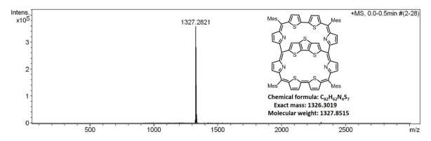
Figure 5.18: ESI-MS spectrum of 30a
