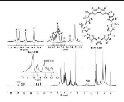
Figure 6.14: <sup>1</sup>H NMR spectrum of 17b.2H<sup>+</sup> in CD<sub>2</sub>Cl<sub>2</sub>. (Inset shows the expansion in
