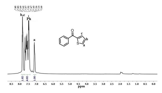
Figure 2.3.11: <sup>1</sup>H NMR spectrum of 19 in CDCl<sub>3</sub>.
