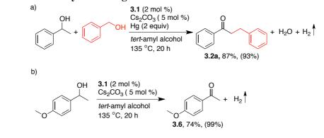
Scheme 3.3 Mercury Poisoning Test and Observation of Ketone Intermediate
