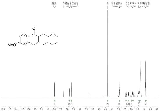
**Figure 3.15** <sup>1</sup>H NMR spectrum of 6-methoxy-2-octyl-3,4-dihydronaphthalen-1(2H)-one **(3.5c**):
