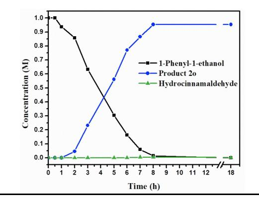
In a further attempt to identify the intermediates involved in this transformation, the catalytic reaction of 1-phenyl-1-ethanol with benzyl alcohol was intervened and the reaction mixture was subjected to <sup>1</sup>H NMR analysis, which resonated a characteristic singlet at  $\delta$  10.05 ppm and a distinct doublet at  $\delta$  7.85 ppm with a coupling constant *J* = 16 Hz that corresponds to aldehyde proton of benzaldehyde and olefin protons of E-chalcone, respectively.<sup>64</sup>
