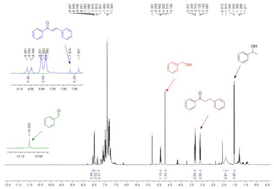
**Figure 3.19** <sup>1</sup>H NMR Spectrum of Reaction Mixture **3.2a**: Observation of Aldehyde and  $\alpha,\beta$ –Unsaturated Ketone Intermediates
