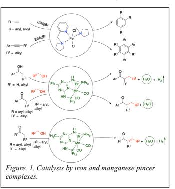
hydrogen are the only byproduct in these catalytic processes. Mechanistic studies indicated that these catalytic transformations proceed through O–H bond activation of alcohols via dearomatization–aromatization metal-ligand cooperation operative in catalysts leading to the oxidation of alcohols.
