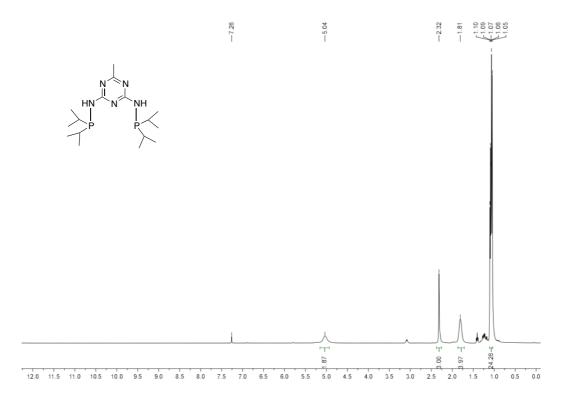
Figure 4.6 <sup>1</sup>H NMR spectrum of  $[(4-Me)Tr(NHP(^{i}Pr)_2)_2Mn(CO)_2Br]$  (Catalyst 4.1):
