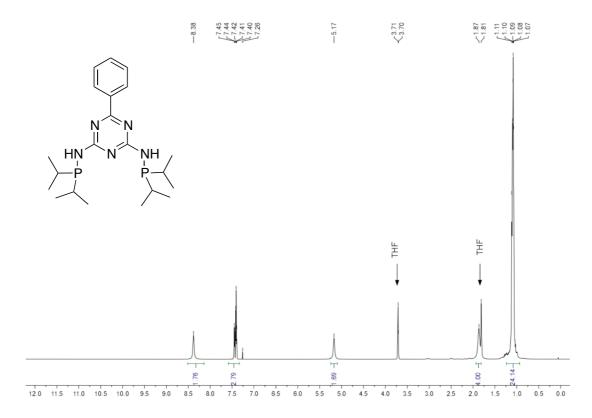
Figure 4.2 <sup>1</sup>H NMR spectrum of  $(4-Ph)Tr(NHP(iPr)_2)_2$  (L4):
