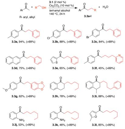
Table 3.3 Manganese-Catalyzed α-Alkylation of Ketones Using Alcohols<sup>a</sup>
