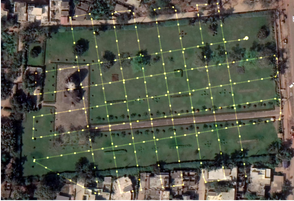
Fig. 6.7: UAV flight path for photogrammetric data acquisition. The yellow dots indicate photograph capture positions, with the larger dot marking the starting location. The flight pattern follows a systematic grid at 80m altitude with 75% forward and side overlap, ensuring complete coverage of the temple complex. Base imagery courtesy of Google Maps.
