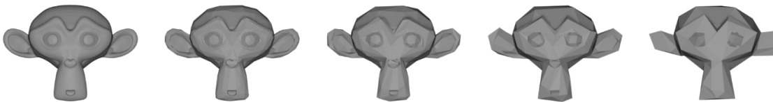
Fig. 6.11: Progressive decimation on a simplified mesh geometry. Each step removes 50% of vertices through edge contraction. The sequence demonstrates how mesh topology simplifies while maintaining approximate surface shape.
